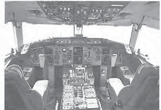
FIGURE 13.3 The flight deck of the Boeing 757 and 767 features digital control electronics, including an engine indicating system and a crew alerting system. All systems controls are within reach of either pilot. The system includes an inertial reference system making use of laser gyroscopes and an electronic attitude director indicator. A flight-management computer system integrates navigation, guidance, and performance data functions. When coupled with the automatic flight control system, the flight-management system provides accurate engine thrust settings and flight-path guidance during all phases of flight from immediately after takeoff to final approach and landing. (Courtesy of Boeing Airplane Co.)
