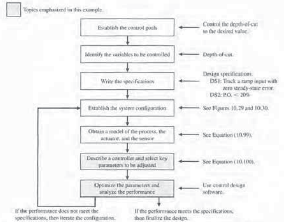
FIGURE 10.31 Elements of the control system design process emphasized in this milling machine control system design example.
