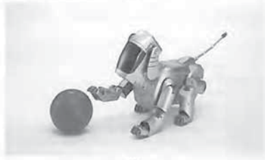
FIGURE 13.15 (a) Aibo is a sophisticated entertainment robot. Aibo looks like a Chihuahua and wags its tail, does tricks, and goes for walks. Aibo depends on a wide range of sensors, including touch, color CCD camera, range finder, and velocity sensors. A 64-bit RISC micro-processor and 19MB of memory are built in. It has 18 joints powered by 18 motors. Photo courtesy of Sony Electronics Inc. (b) Feedback control system with a digital controller. (c) Block diagram model. Note that G(z) = Z[G_d(s)G_p(s)] .
