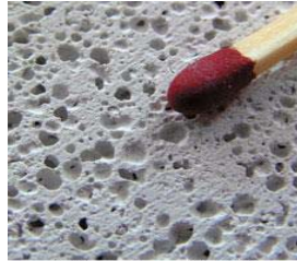
Cellular structure of Hebel AAC
