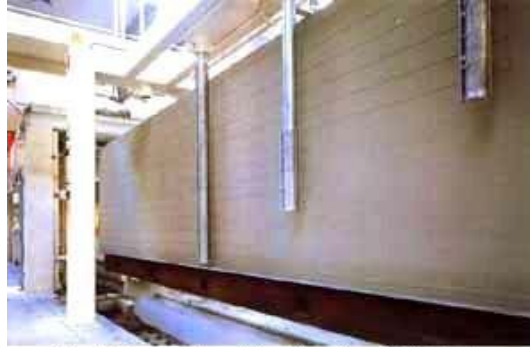
Wire Cutter machine slicing through soft AAC cake
