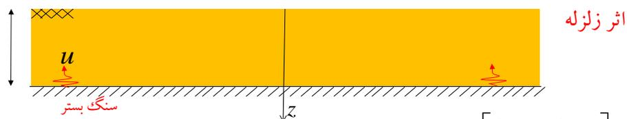
$$u = u_0 \sin[\omega(t - x/c_2)] = u_0 \sin[\omega t - \lambda_2 x] = u_0 \sin\left[\frac{2\pi}{T}t - \frac{2\pi}{l_2}x\right]$$
