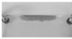
FIGURE 4-1 Demonstration of capillary action. (All illustrations in this chapter courtesy C. J. Hellier.) (a) Glass panes clamped together. (b) Visible color contrast penetrant applied to edge of panes.
