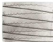
Fig. 4. Type A scanning and timing system. This is the part which operates on the screen when the crystal is not being energized. It operates essentially by the zero spot of the oscilloscope traveling along the oblique path A, B, C, D, etc. Each slightly elevated or depressed spot in the wave is detected. The line scan thereby forms a strong scale. Every amplitude variation is made higher in order to assist in measuring. There are other methods, higher resolution systems, and that is reserved for fiberoptic or laser-scatter imaging.
