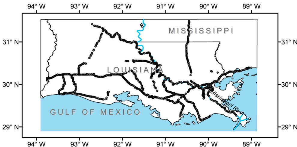
Fig. 1 Plot of the network of benchmarks used for interpolation of rates of vertical displacement in the selected area
