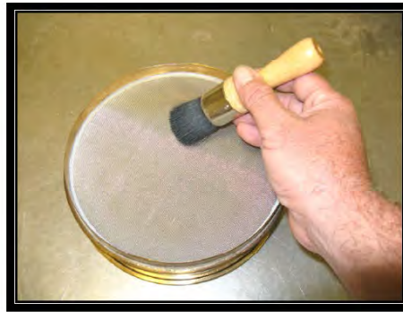
Figure 4 Use Hair Brush on Fine Sieves
