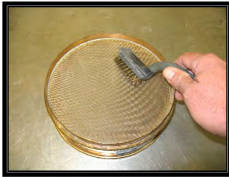
Figure 3 Use Wire brush on Coarse Sieve
