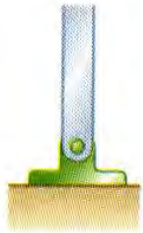
Frictionless pin or hinge
