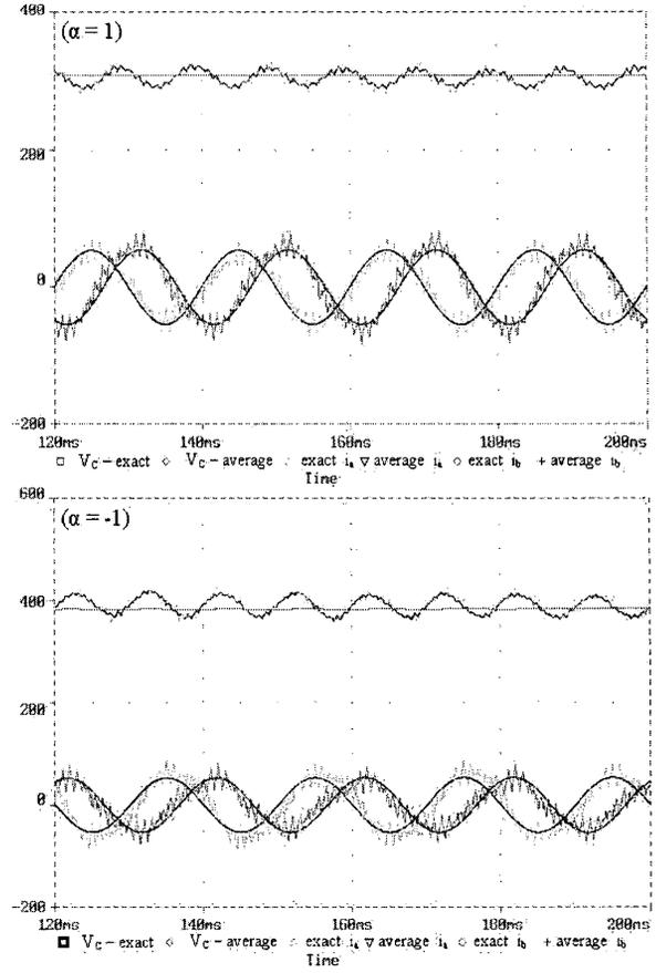
Figure 4: Results of the average equivalent circuit model simulated with PSpice: (a)  $\alpha = 1^\circ$  (inductive); (b)  $\alpha = -1^\circ$  (capacitive).
