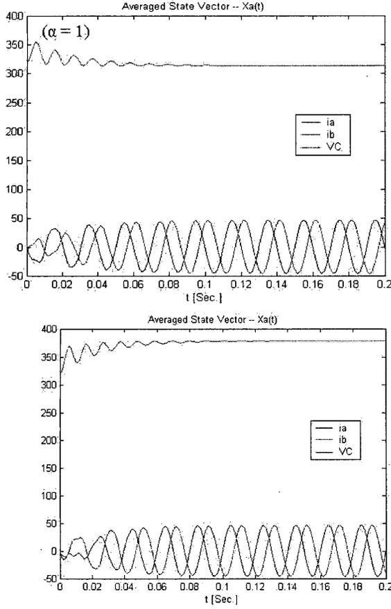
Figure 3: MATLAB simulation results for the average model, two cases: (a)  $\alpha = 1^\circ$  (inductive); (b)  $\alpha = -1^\circ$  (capacitive).
