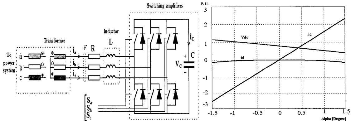
Figure 1: (a) An equivalent three-phase circuit of STATCOM; (b) equivalent reactive current, active current, and capacitor voltage as a function of  $\alpha$ .
