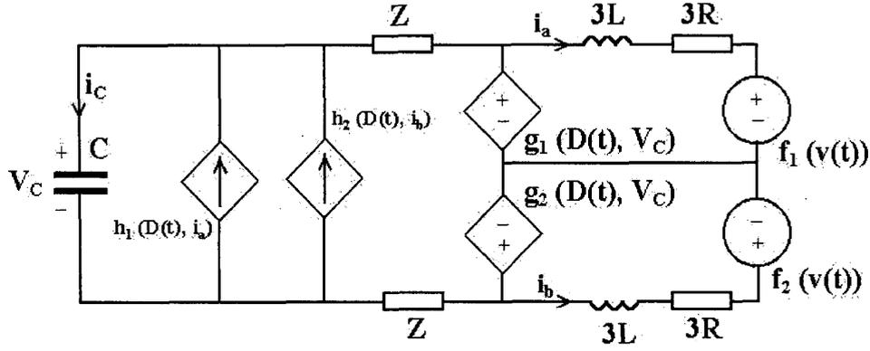
Figure 2: Equivalent circuit average model of STATCOM, suitable for circuit simulators such as SPICE.
