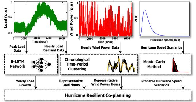
Fig. 5. The structure of the proposed method to handle the uncertainties
