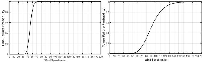
Fig. 2. The Fragility Curves of line (left) and tower (right)
