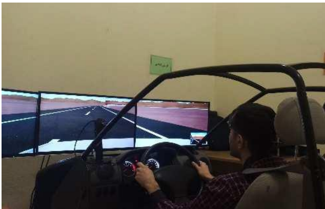
Fig. 4. Simulator during the experiment; The camera located on the left side of the steering wheel captures the driver's face and neck while not disrupting their view of the screen for the driver
