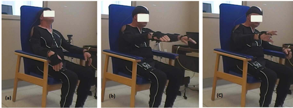
Fig. 1. All participants were asked to perform three standard tasks: (a) Rest, (b) Posture, and (c) Action while seated, wearing IGS-180 motion capture suit.
