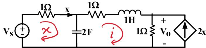
$$\left\{ \begin{array}{l} V_s = 1X + \frac{1}{s}(X - I) \\ I + sI + 1(2X + I) + \frac{1}{s}(I - X) = 0 \end{array} \right. \rightarrow \left\{ \begin{array}{l} (1 + \frac{1}{s})X - \frac{1}{s}I = V_s \\ (2 - \frac{1}{s})X + (2 + s + \frac{1}{s})I = 0 \end{array} \right. \rightarrow X = \frac{s^2 + 4s + 1}{1 - 4s} I \rightarrow$$
