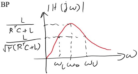
$$|H(j\omega)| = \frac{L\omega}{\sqrt{(R - \gamma RLC\omega^2)^2 + (R^2C + L)^2\omega^2}} = \frac{L}{(R^2C + L)\sqrt{\gamma}} \rightarrow (R - \gamma RLC\omega^2) = \pm (R^2C + L)\omega \rightarrow$$
