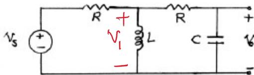
$$\frac{V_o}{V_s} = \frac{\frac{1}{Cs}}{R + \frac{1}{Cs}} = \frac{1}{1 + RCs}, \quad \frac{V_1}{V_s} = \frac{Z}{Z + R} \quad Z = Ls \parallel \left(R + \frac{1}{Cs}\right) = \frac{Ls\left(R + \frac{1}{Cs}\right)}{Ls + R + \frac{1}{Cs}} = \frac{Ls(1 + RCs)}{LCs^2 + RCs + 1} \rightarrow$$
