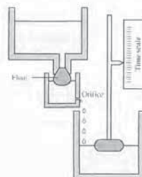
FIGURE P1.11 Water clock. (From Newton, Gould, and Kaiser, Analytical Design of Linear Feedback Controls , Wiley, New York, 1957, with permission.)
