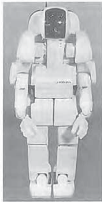
FIGURE 1.11 The Honda P3 humanoid robot. P3 walks, climbs stairs, and turns corners. Photo courtesy of American Honda Motor, Inc.
