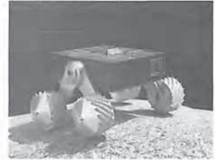
FIGURE P1.26 Micro-rover designed to explore an asteroid. (Photo courtesy of NASA.)
