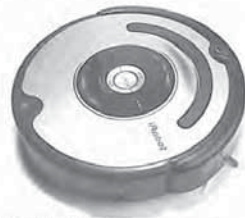
FIGURE AP1.6 A robotic vacuum cleaner communicates with the base station as it maneuvers around the room. (Photo courtesy of Alamy Images.)
