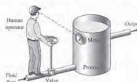
FIGURE P1.2 Fluid-flow control.
