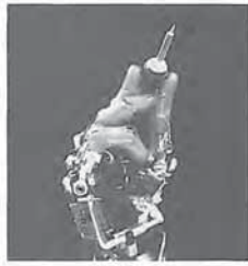
FIGURE 4.16 The DLR German Aerospace Center is developing an advanced robotic hand. The final goal—fully autonomous operation—has not yet been achieved. Currently, the control is accomplished via a telemanipulation system consisting of a lightweight robot with a four-fingered articulated hand mounted on a mobile platform. The hand operator receives stereo video feedback and force feedback. This information is employed in conjunction with a data glove equipped with force feedback and an input device to control the robot. (Used with permission. Credit: DLR Institute of Robotics and Mechatronics.)
