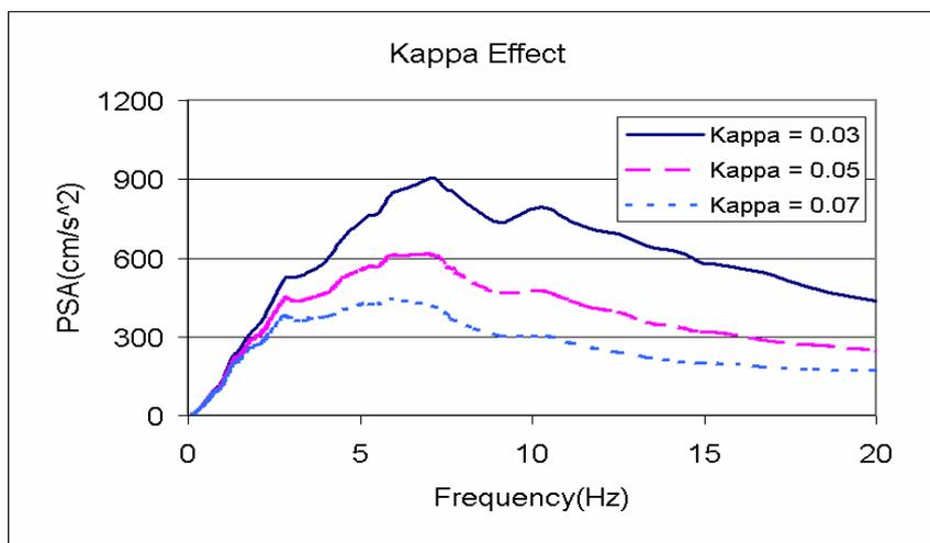
Figure 4 Simulated spectral accelerations for different values of  $\kappa$
