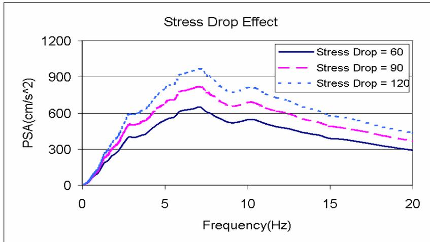
Figure 5 Simulated spectral accelerations for different values of  $\Delta\sigma$
