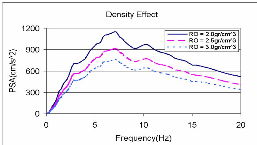
Figure 7 Simulated spectral accelerations for different values of  $\rho$
