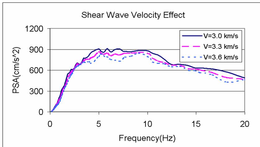
Figure 6 Simulated spectral accelerations for different values of  $\beta$
