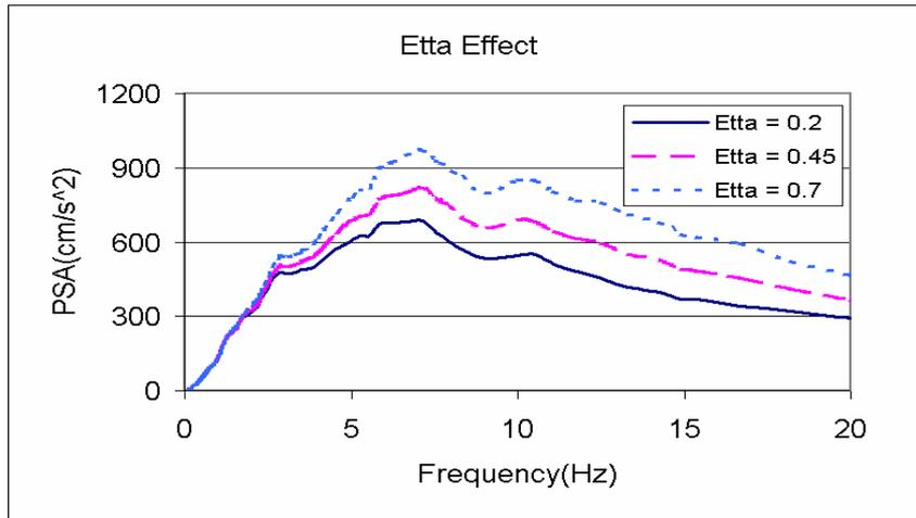
Figure 2 Simulated spectral accelerations for different values of  $\eta$
