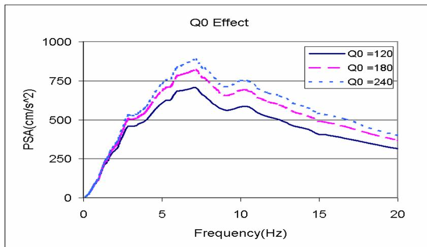
Figure 1 Simulated spectral accelerations for different values of  $Q_0$
