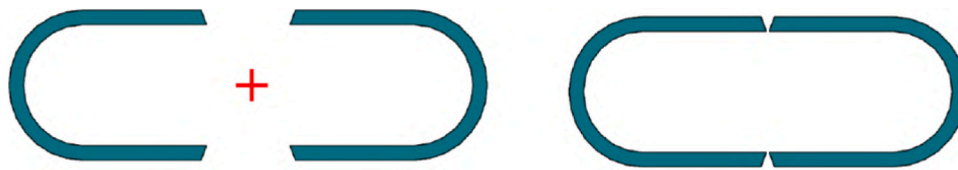
Fig. 1. Combination of Two U-Shaped Dampers and the Construction of an Elliptical Damper.
