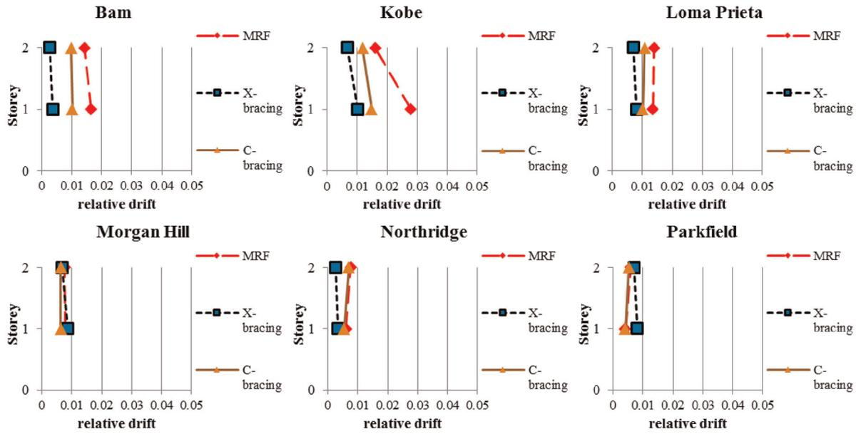
Figure 16. Relative drift of storeys of two-storey frames for PGA = 0.35g.
