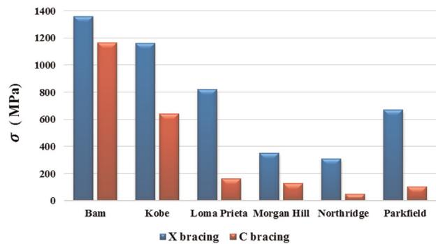
**Figure 33.** Maximum stress of bracing cables of six-storey frames for PGA = 0.50g.
