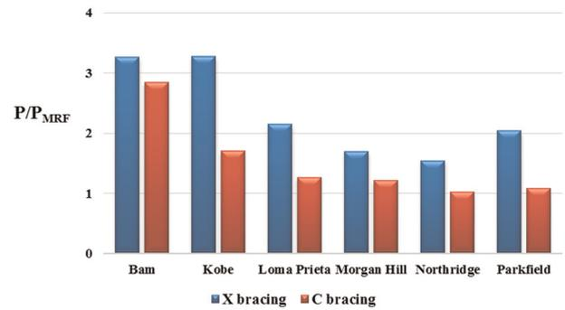
**Figure 27.** Ratio of braced frame column force of strengthened frames to the column force of MRFs in six-storey frames for PGA = 0.50g.
