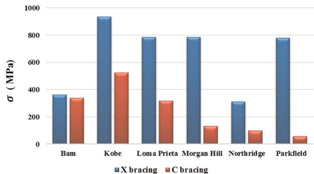
**Figure 28.** Maximum stress of bracing cables of two-storey frames for PGA = 0.35g.
