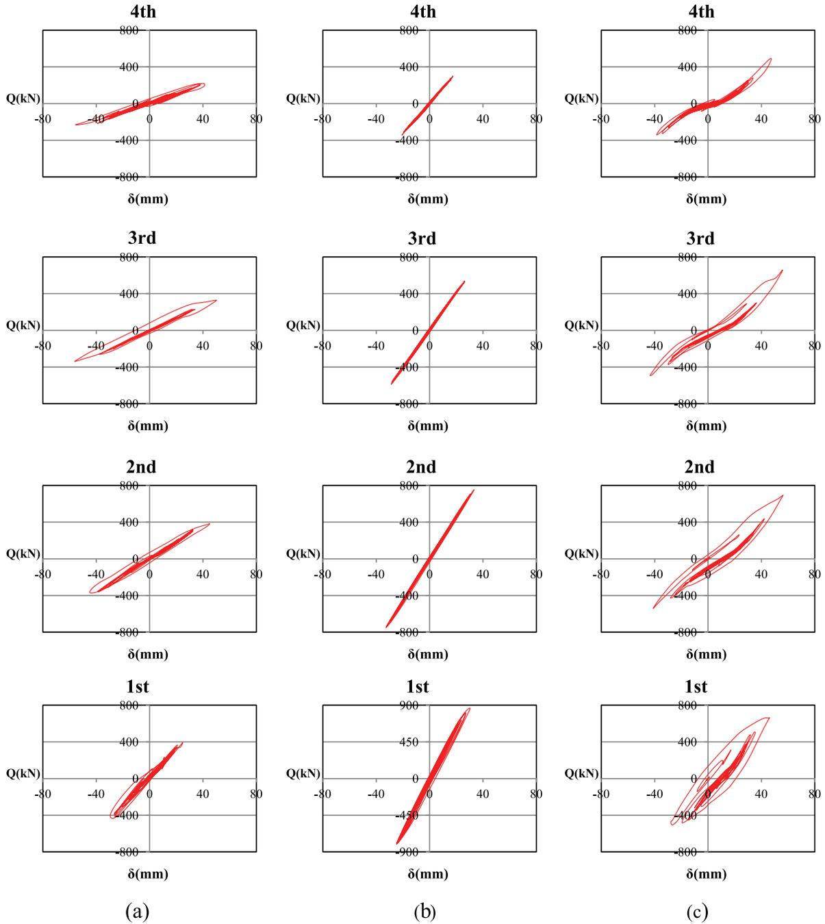
**Figure 12.** Hysteresis curves of four-storey frames subjected to Cobe earthquake record with PGA = 0.35g: (a) MRF, (b) MRF with cable cross-bracing and (c) MRF with cable-cylinder bracing.
