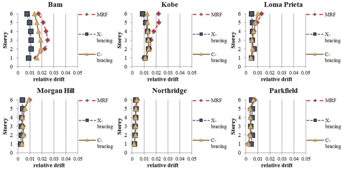
Figure 20. Relative drift of storeys of six-storey frames for PGA = 0.35g.
