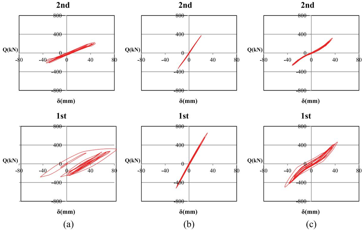
**Figure 10.** Hysteresis curves of two-storey frames subjected to Cobe earthquake record with PGA = 0.35g: (a) MRF, (b) MRF with cable cross-bracing and (c) MRF with cable-cylinder bracing.
