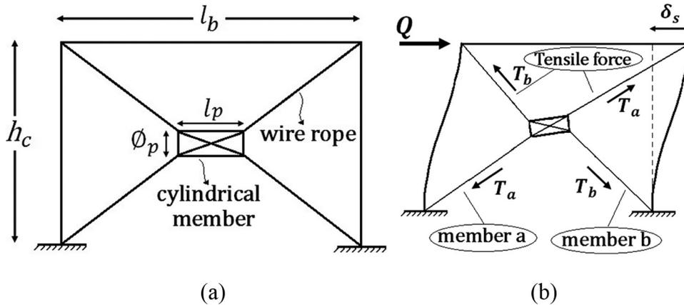
**Figure 1.** Cable bracing system with central cylinder: (a) dimensions and (b) deformation at  $\delta_s$ .
