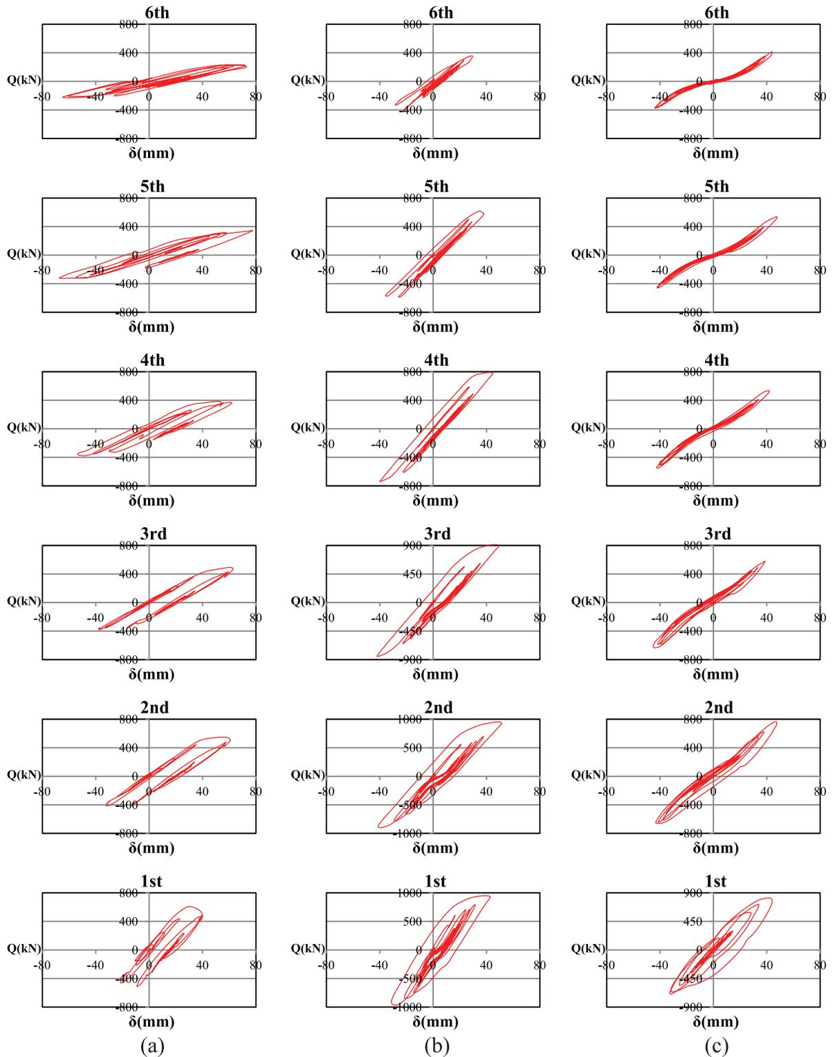
**Figure 15.** Hysteresis curves of six-storey frames subjected to Cobe earthquake record with PGA = 0.50g: (a) MRF, (b) MRF with cable cross-bracing and (c) MRF with cable-cylinder bracing.
