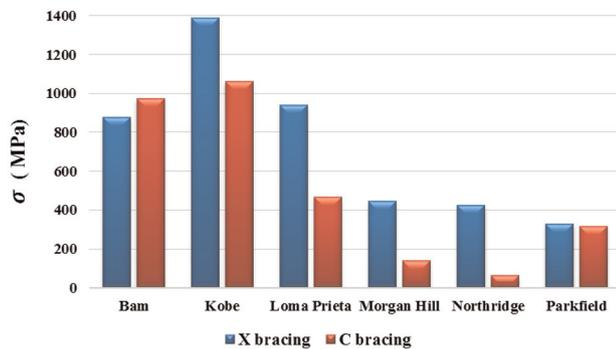
**Figure 31.** Maximum stress of bracing cables of four-storey frames for PGA = 0.50g.
