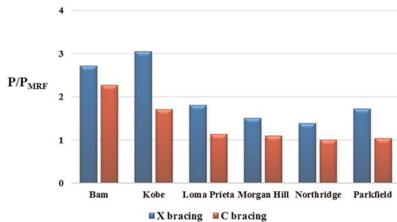
**Figure 26.** Ratio of braced frame column force of strengthened frames to the column force of MRFs in six-storey frames for PGA = 0.35g.
