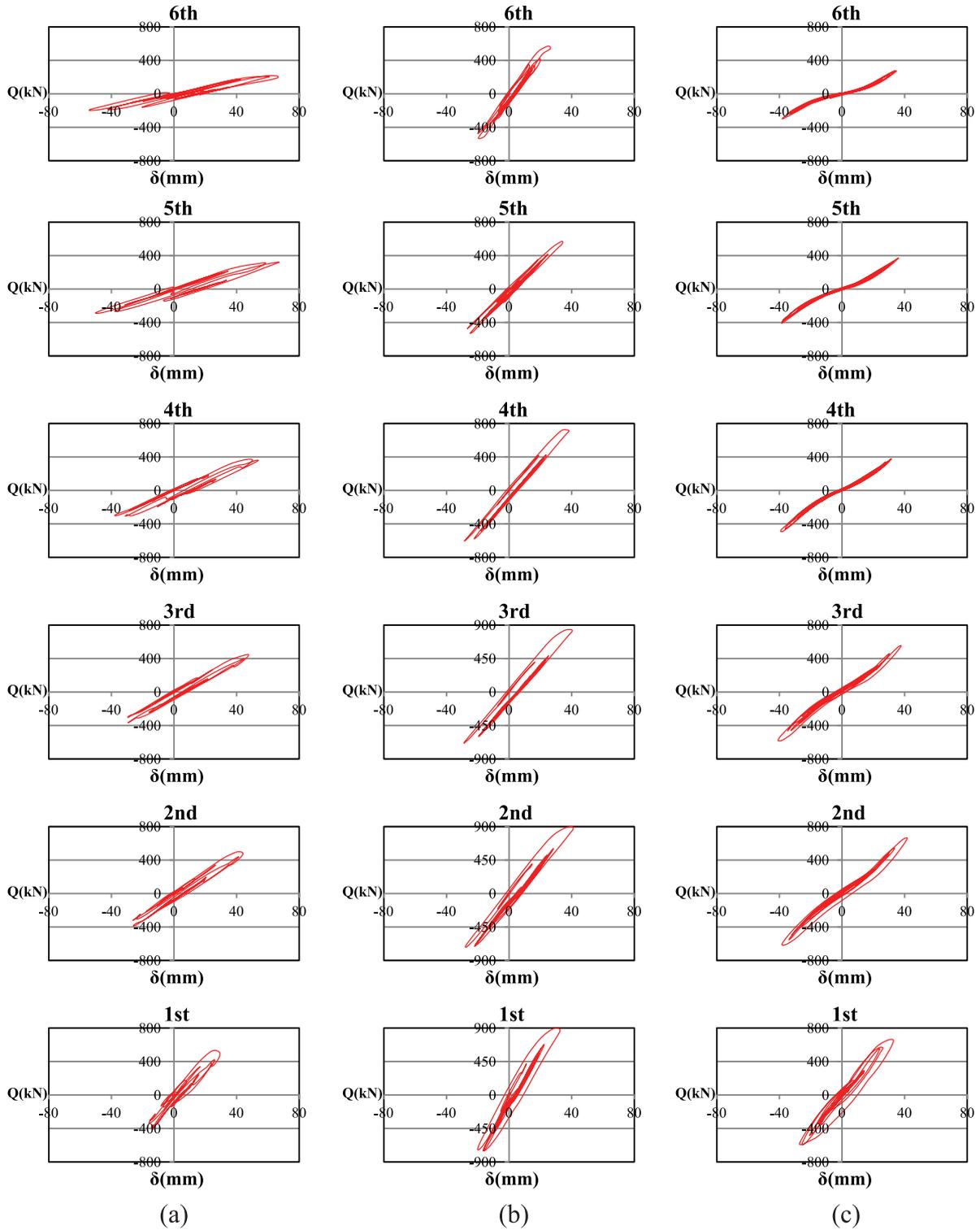
**Figure 14.** Hysteresis curves of six-storey frames subjected to Cobe earthquake record with PGA = 0.35g: (a) MRF, (b) MRF with cable cross-bracing and (c) MRF with cable-cylinder bracing.
