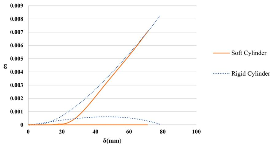
**Figure 9.**  $\epsilon$ - $\delta$  curves for rigid cylinder and the cylinder with the modulus of elasticity equal to 0.001 times of steel.
