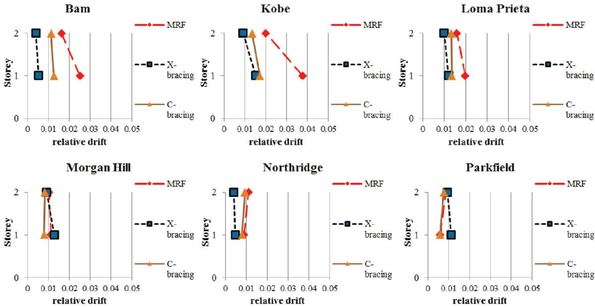
Figure 17. Relative drift of storeys of two-storey frames for PGA=0.50g.
