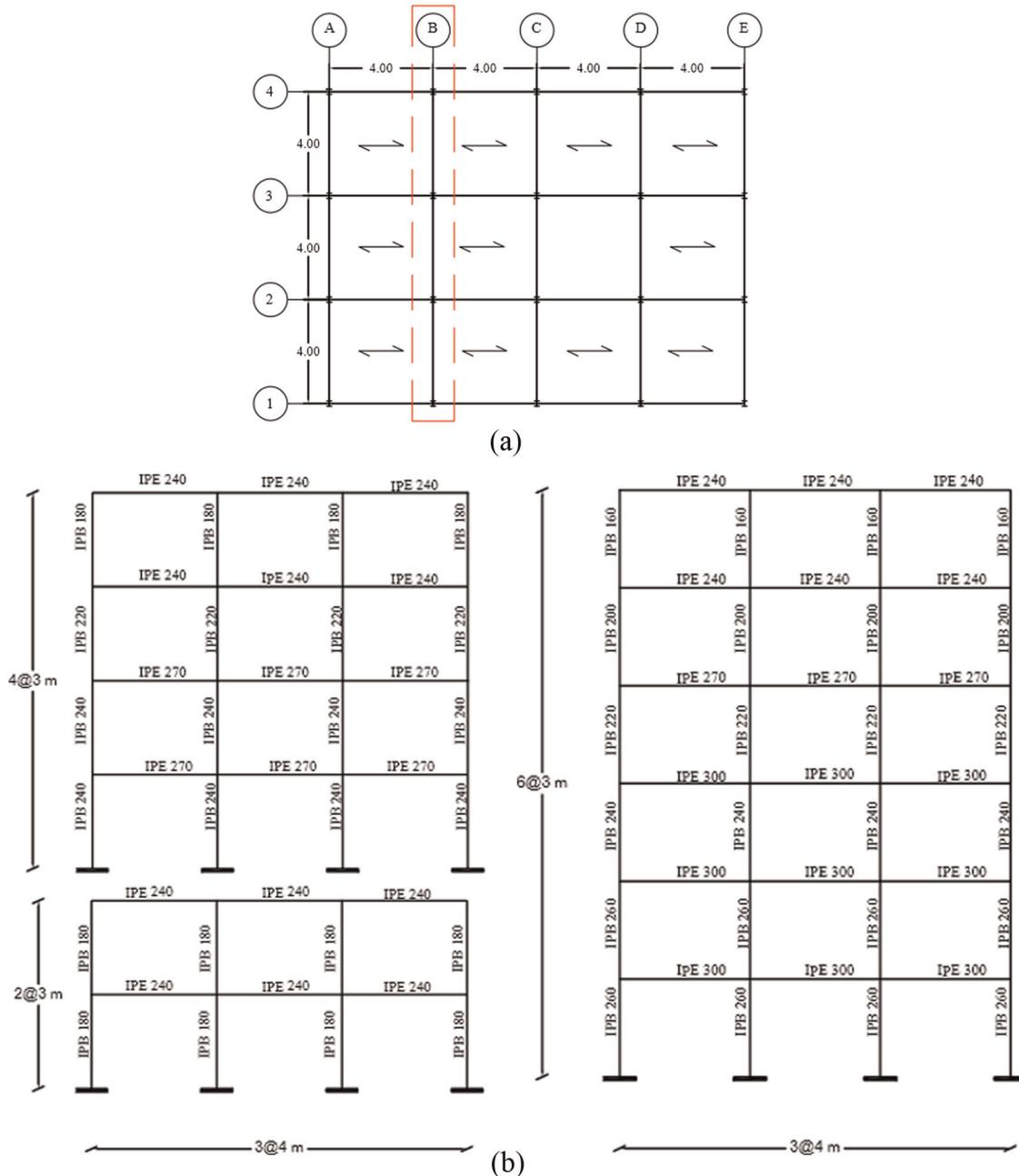
**Figure 2.** (a) Plan of two-, four- and six-storey MRFs and (b) geometry of extracted two-dimensional frames.
