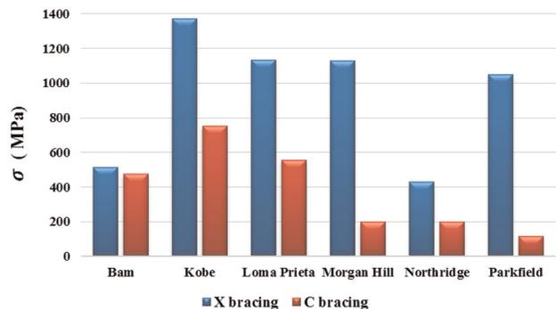
**Figure 29.** Maximum stress of bracing cables of two-storey frames for PGA = 0.50g.
