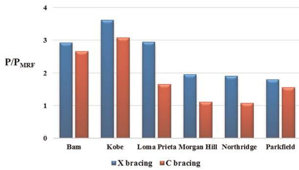
**Figure 25.** Ratio of braced frame column force of strengthened frames to the column force of MRFs in four-storey frames for PGA = 0.50g.
