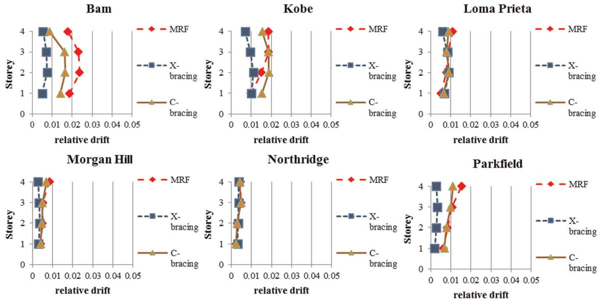
Figure 18. Relative drift of storeys of four-storey frames for PGA = 0.35g.
