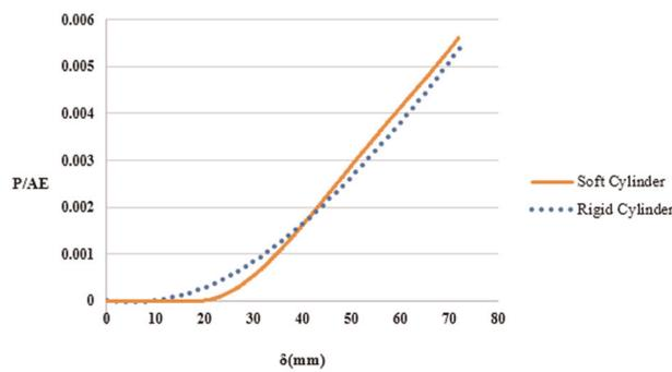
**Figure 8.**  $P$ - $\delta$  curves for rigid cylinder and the cylinder with the modulus of elasticity equal to 0.001 times of steel.
