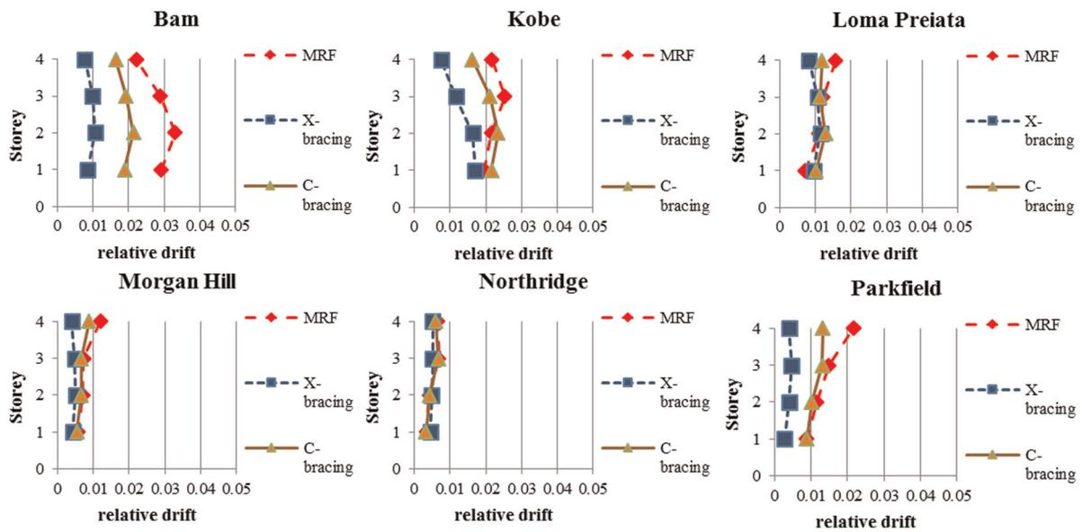
Figure 19. Relative drift of storeys of four-storey frames for PGA = 0.50g.
