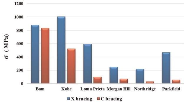
**Figure 32.** Maximum stress of bracing cables of six-storey frames for PGA = 0.35g.
