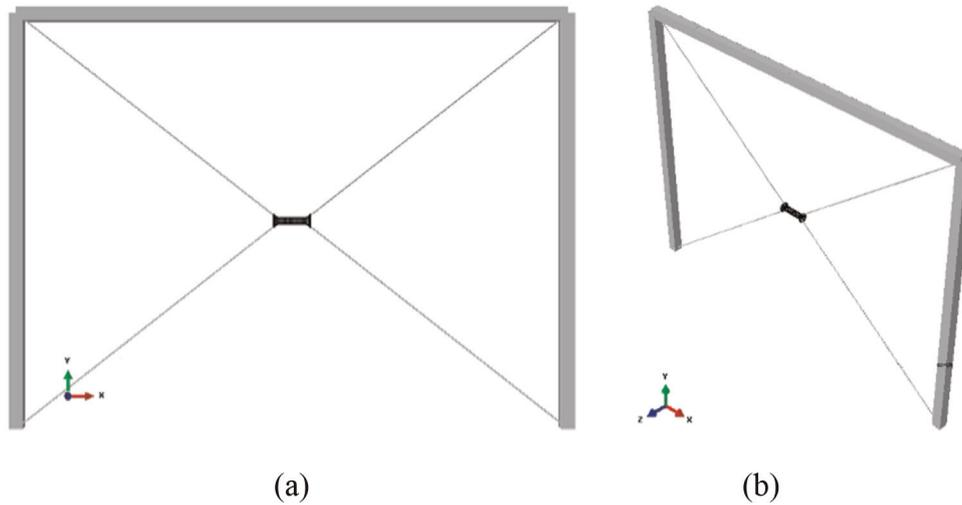
**Figure 5.** FE models of frame with cable–cylinder bracing: (a) front view of 3D model and (b) side view of 3D model.
