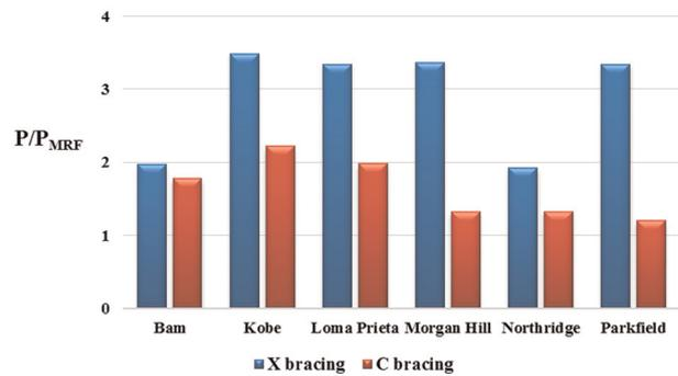
Figure 23. Ratio of braced frame column force of strengthened frames to the column force of MRFs in two-storey frames for PGA = 0.50g.
