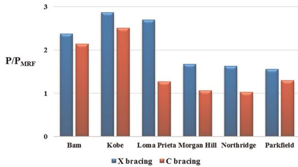
**Figure 24.** Ratio of braced frame column force of strengthened frames to the column force of MRFs in four-storey frames for PGA = 0.35g.
