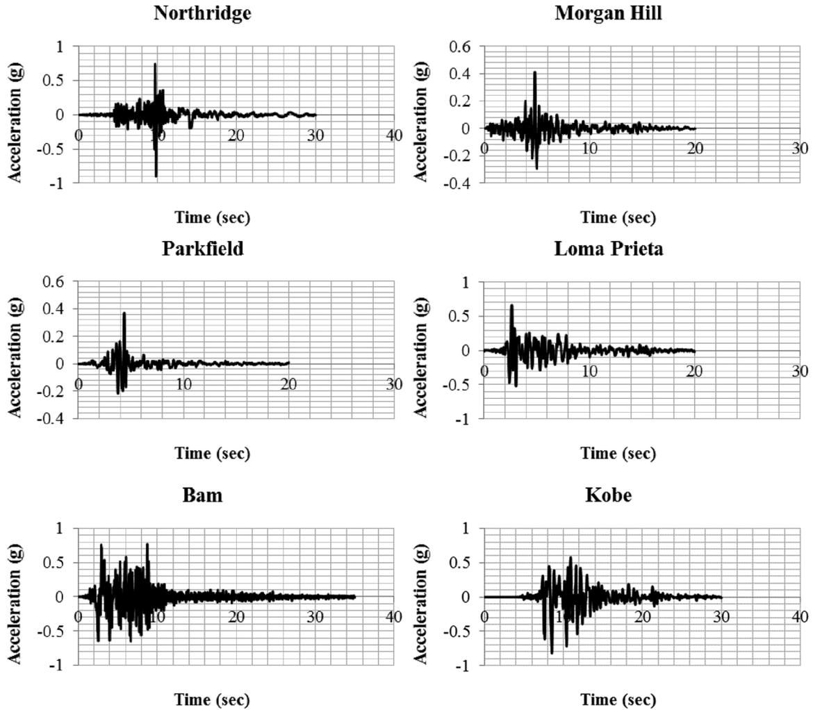
**Figure 4.** Accelerograms used in the seismic analyses.
