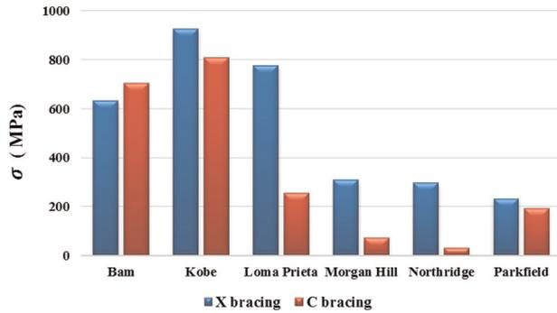
**Figure 30.** Maximum stress of bracing cables of four-storey frames for PGA = 0.35g.
