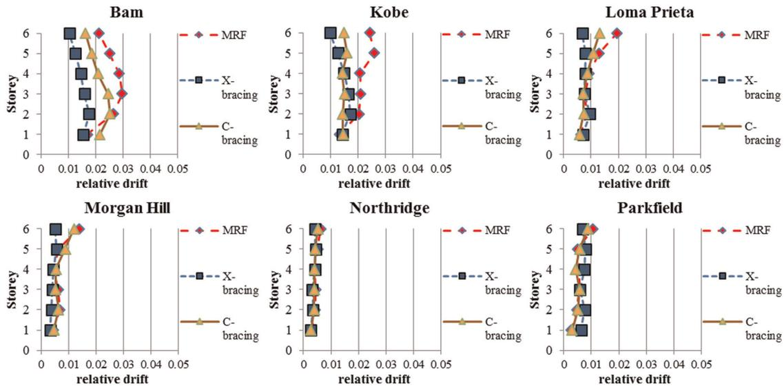
Figure 21. Relative drift of storeys of six-storey frames for PGA = 0.50g.
