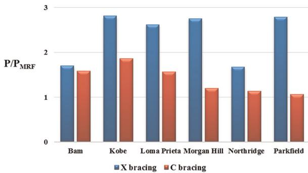
Figure 22. Ratio of braced frame column force of strengthened frames to the column force of MRFs in two-storey frames for PGA = 0.35g.
