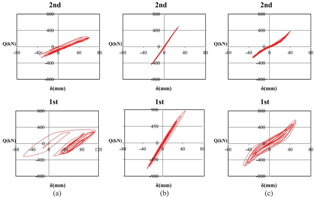
**Figure 11.** Hysteresis curves of two-storey frames subjected to Cobe earthquake record with PGA = 0.50g: (a) MRF, (b) MRF with cable cross-bracing and (c) MRF with cable-cylinder bracing.
