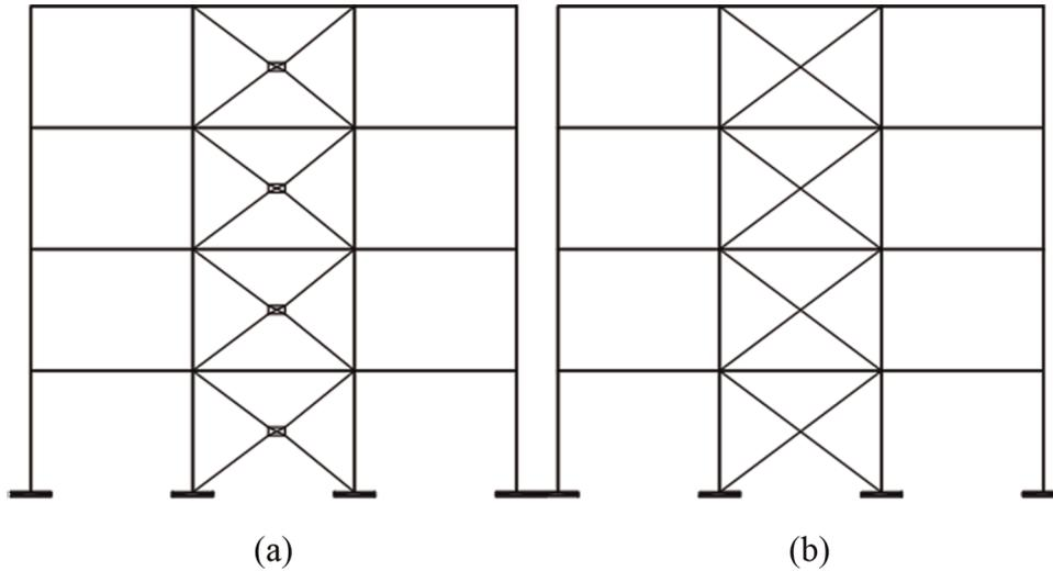
**Figure 3.** Studied structural strengthening systems: (a) cable–cylinder bracing and (b) cable cross bracing.
