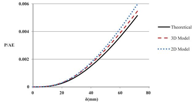
**Figure 6.** The  $P$ – $\delta$  curves of theoretical relations and numerical modelling.
