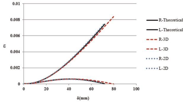
**Figure 7.** The  $\epsilon$ - $\delta$  curves of theoretical relations and numerical modelling.
