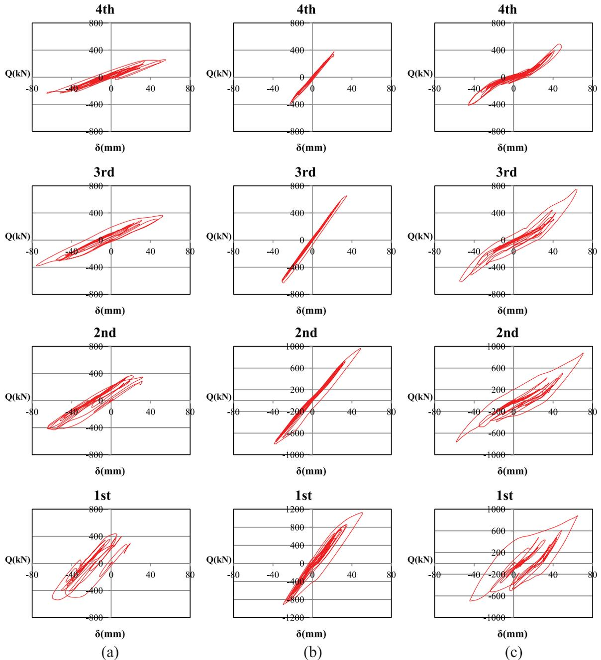
**Figure 13.** Hysteresis curves of four-storey frames subjected to Cobe earthquake record with  $PGA = 0.50g$ : (a) MRF, (b) MRF with cable cross-bracing and (c) MRF with cable-cylinder bracing.
