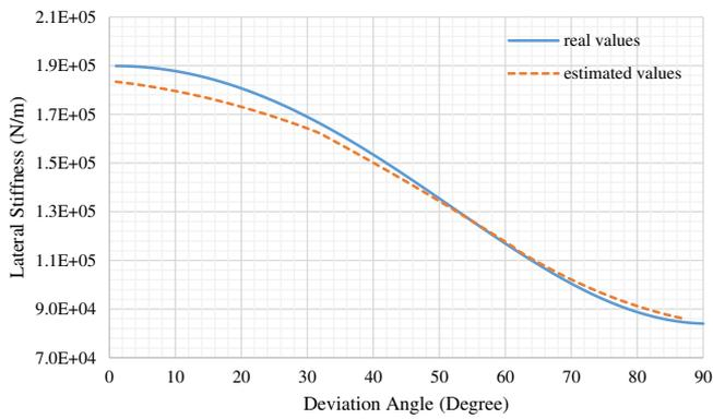
Fig. 27. The values obtained from the explained equations and real values for the sixth case.
