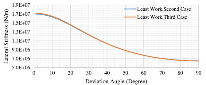
Fig. 15. Lateral stiffness of the steel frame in the second and third cases.
