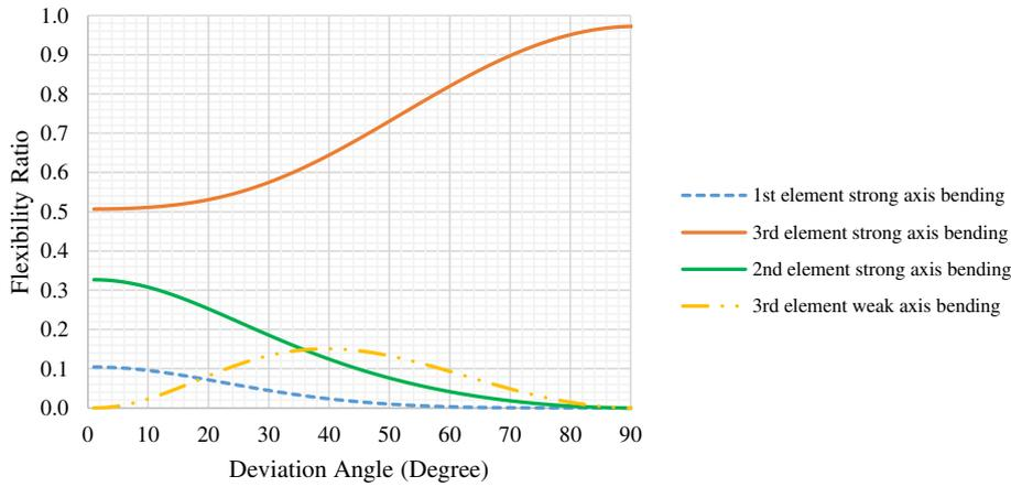
Fig. 22. Cooperation rate of internal efforts in the lateral flexibility of the steel frame in the sixth case.
