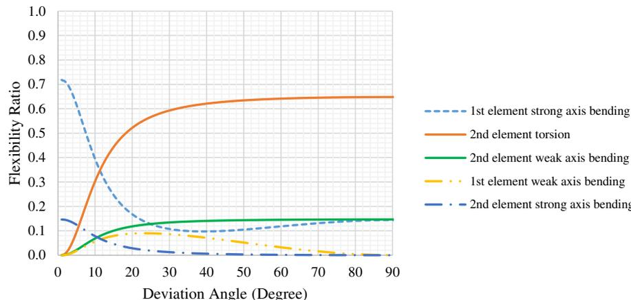
Fig. 21. Cooperation rate of internal efforts in the lateral flexibility of the steel frame in the fifth case.
