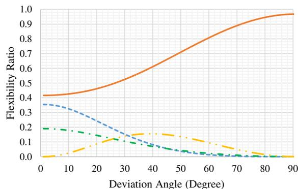
Fig. 19. Cooperation rate of internal efforts in the lateral flexibility of the steel frame in the third case.
