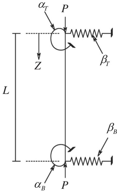
Fig. 3. The boundary conditions considered for the element under buckling.
