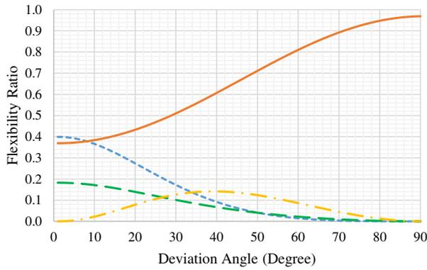
Fig. 18. Cooperation rate of internal efforts in the lateral flexibility of the steel frame in the second case.
