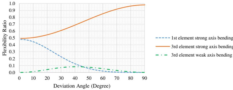
Fig. 20. Cooperation rate of internal efforts in the lateral flexibility of the steel frame in the fourth case.
