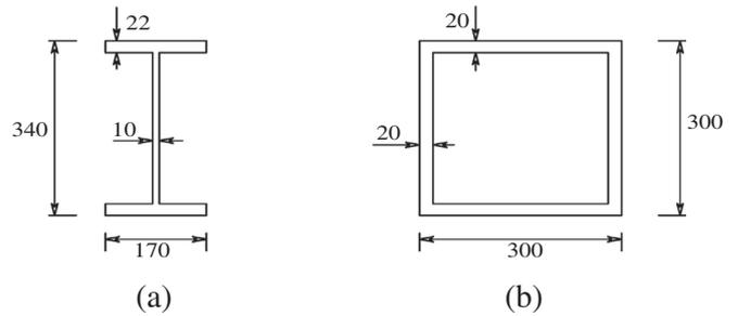
Fig. 13. The sections used for a) beam and b) columns, the values as per mm.
