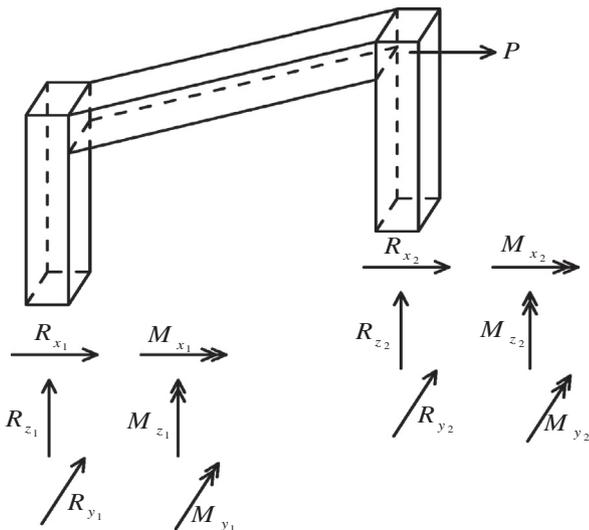
Fig. 11. Lateral load applied to the steel frame and the supporting reactions.
