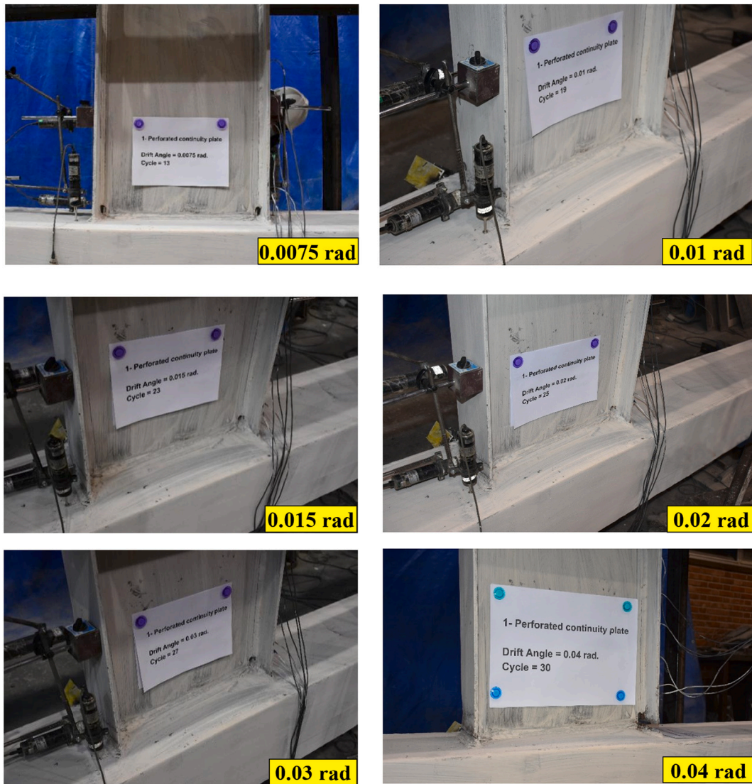
Fig. 12. Status of specimen 1 (ID) during different loading cycles.
