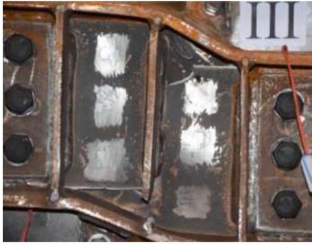
Fig. 2. Fracture in the vicinity of stiffener connection to the link beam web [7].
