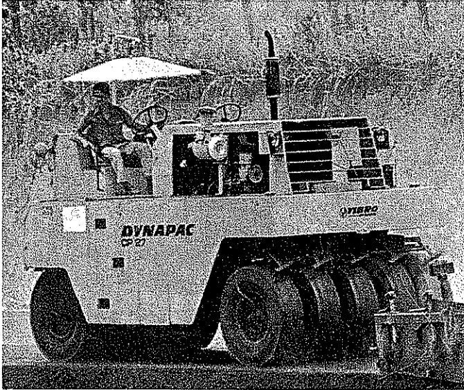
Figure 9.18. Pneumatic tired roller for the compaction of slightly cohesive soils (courtesy of Dynapac).
