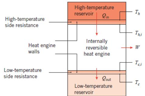
Internally reversible heat engine exchanging heat with high- and low-temperature reservoirs through thermal resistances
