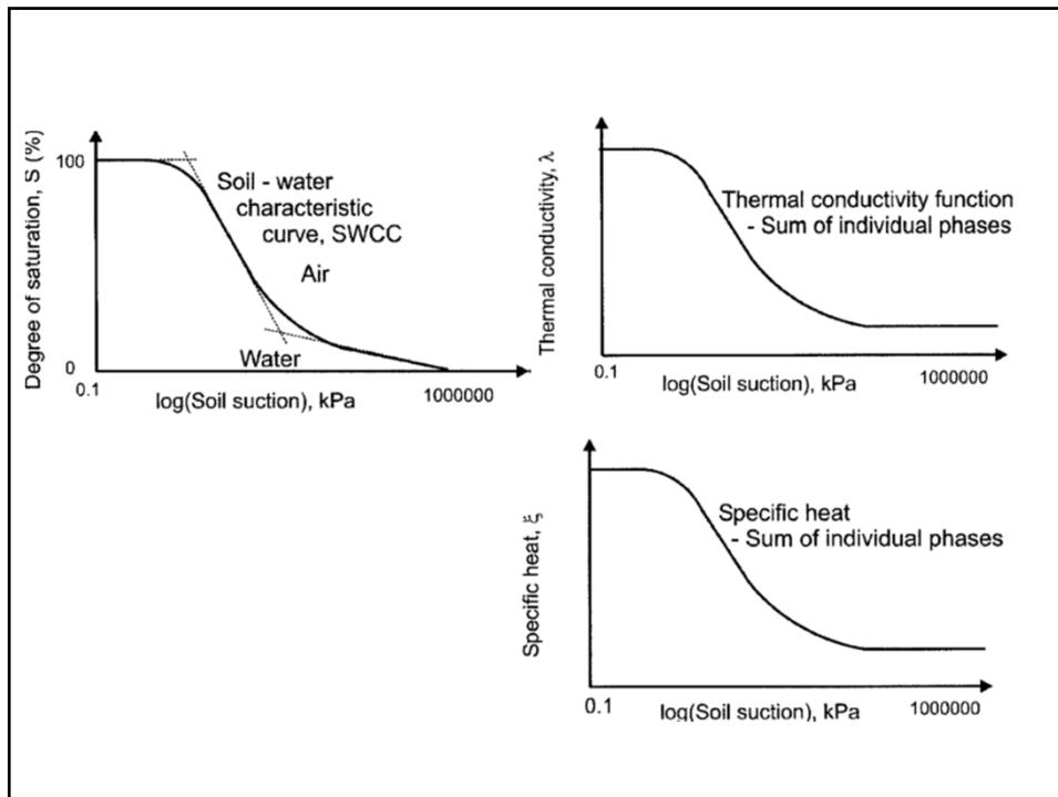
**Table 7.** Functions for Heat Capacity and Thermal Conductivity of an Unsaturated Soil
