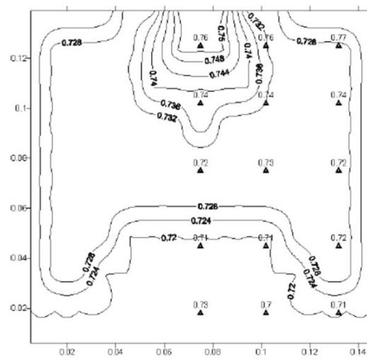
Fig. 5 Experimental (Villar et al., 1993) and calculated void ratio
