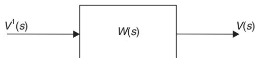
Fig. 9.22 Transformation of a normalized bounded input V^1(s) into an actual input V(s) .
