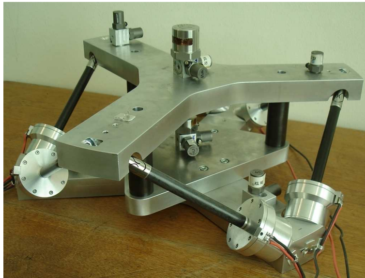
Fig. 8.19. Multi-purpose soft isolator based on a Gough-Stewart platform with cubic architecture (ULB).
