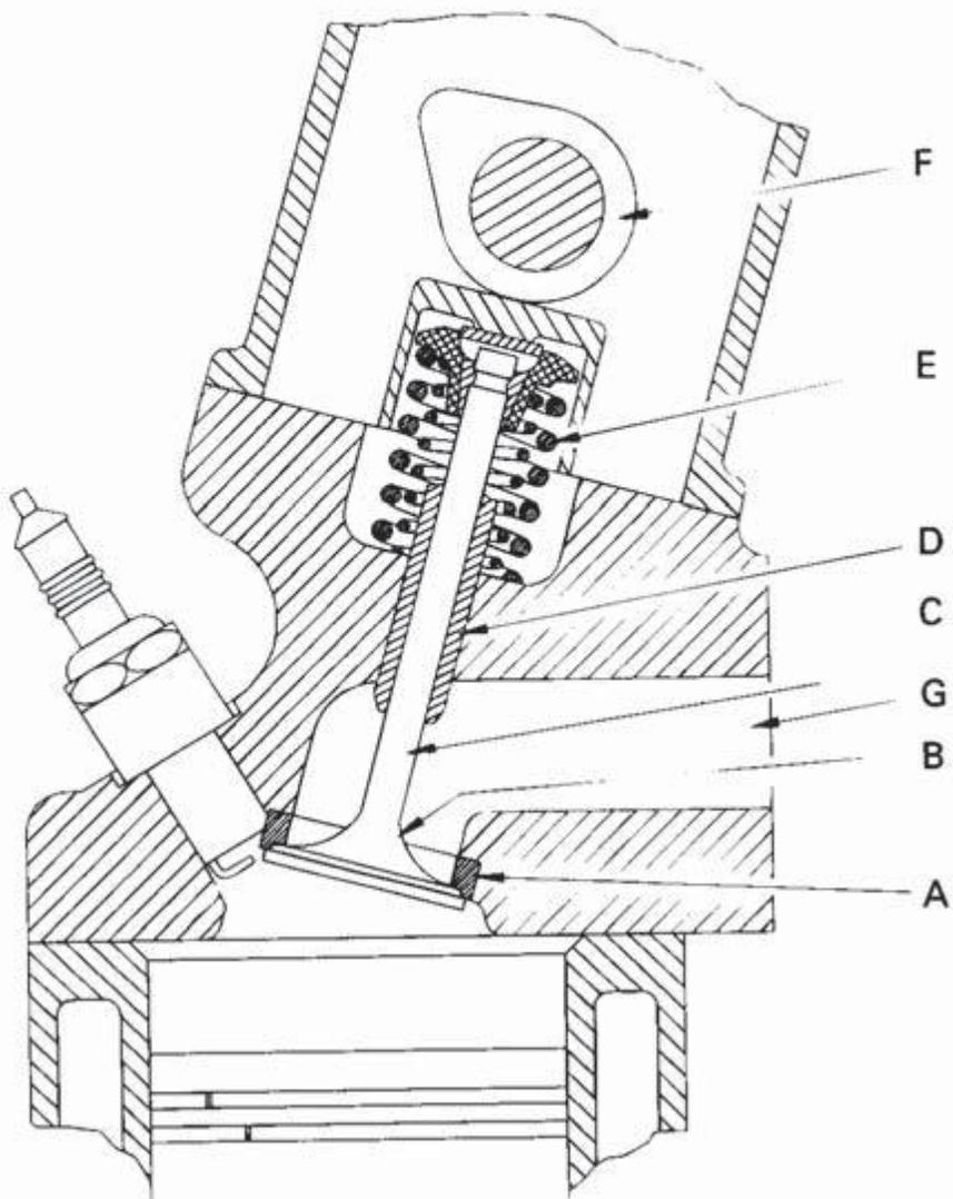
Poppet valve is spring loaded closed, and pushed open by cam action at proper time in cycle. Most automobile engines and other reciprocating engines use poppet valves. Much less common are sleeve valves and rotary valves. Components include: (A) valve seat, (B) head, (C) stem, (D) guide, (E) spring, (F) camshaft, (G) manifold
