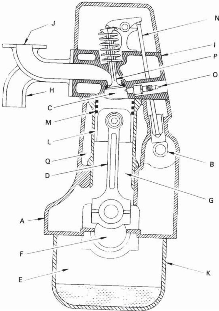
**Figure 1-15** Cross-section of four-stroke cycle S1 engine showing engine components; (A) block, (B) camshaft, (C) combustion chamber, (D) connecting rod, (E) crankcase, (F) crankshaft, (G) cylinder, (H) exhaust manifold, (I) head, (J) intake manifold, (K) oil pan, (L) piston, (M) piston rings, (N) push rod, (O) spark plug, (P) valve, (Q) water jacket.
