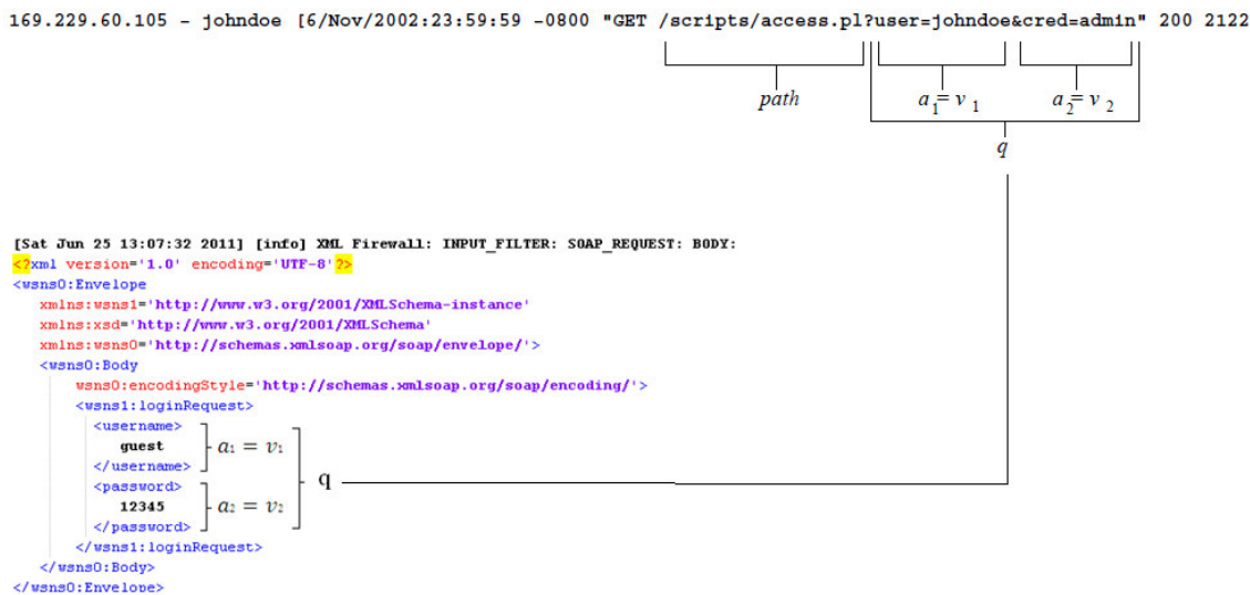
Figure 2- Different Between Web Service Model and Web Model
