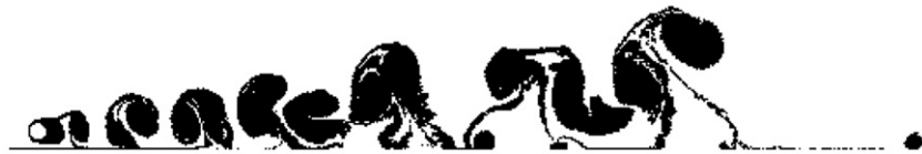
Fig. 19. Final position of the vortices for the flow past a circular cylinder in moving ground for h/d=0.45 at Reynolds number of 1.0 \times 10^5 .
