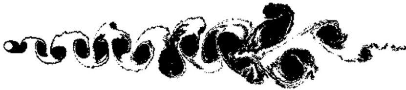
Fig. 18. Final position of the vortices for the flow past an isolated circular cylinder at Reynolds number of 1.0 \times 10^5 .
