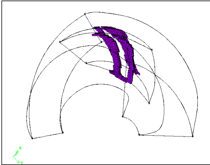
Figure 10-10: Hexahedral mesh elements—EquiAngle Skew = 0.2–0.3
