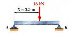
$$\sum M_B = 0: -A_y(6 \text{ m}) + (18 \text{ kN})(6 \text{ m} - 3.5 \text{ m}) = 0$$
