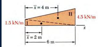
• The line of action of the concentrated load passes through the centroid of the area under the curve.
