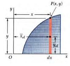
$\overline{x}A = \int \overline{x}_{el} dA$  $= \int x (ydx)$  $\overline{y}A = \int \overline{y}_{el} dA$  $= \int \frac{y}{2} (ydx)$
