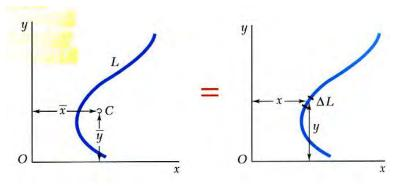
$\overline{x}W = \int x \, dW$   $\overline{x}(\gamma A t) = \int x (\gamma t) dA$   $\overline{x}A = \int x \, dA = Q_y$ = first moment with respect to y  $\overline{y}A = \int y \, dA = Q_x$ = first moment with respect to x
