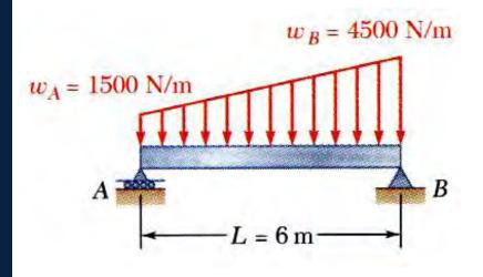
A beam supports a distributed load as shown. Determine the equivalent concentrated load and the reactions at the supports.
