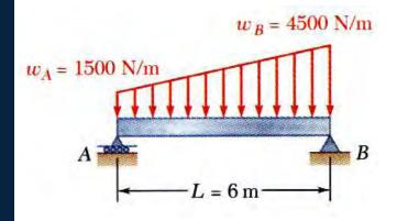
• Determine the support reactions by summing moments about the beam ends.
