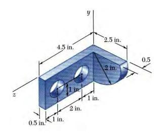
• Moment of the total weight concentrated at the center of gravity G is equal to the sum of the moments of the weights of the component parts.
