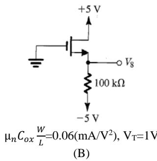
$$\mu_n C_{ox} \frac{W}{L} = 0.06(\text{mA/V}^2), V_T = 1\text{V}$$
