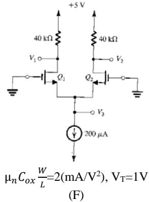
$$\mu_n C_{ox} \frac{W}{L} = 2(\text{mA/V}^2), V_T = 1\text{V}$$
