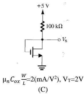
$$\mu_n C_{ox} \frac{W}{L} = 2(\text{mA/V}^2), V_T = 2\text{V}$$
