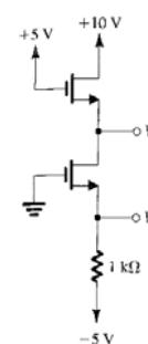
$$\mu_n C_{ox} \frac{W}{L} = 4(\text{mA/V}^2), V_T = 2\text{V}$$
