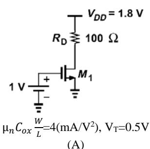
$$\mu_n C_{ox} \frac{W}{L} = 4(\text{mA/V}^2), V_T = 0.5\text{V}$$
