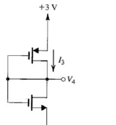
$$\mu_p C_{ox} \frac{W}{L} = 2(\text{mA/V}^2), \mu_n C_{ox} \frac{W}{L} = 2(\text{mA/V}^2), |V_T| = 1\text{V}$$
