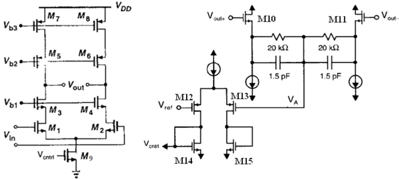
$$V_A = V_{CM} - V_{eff10} - V_{tn}$$
