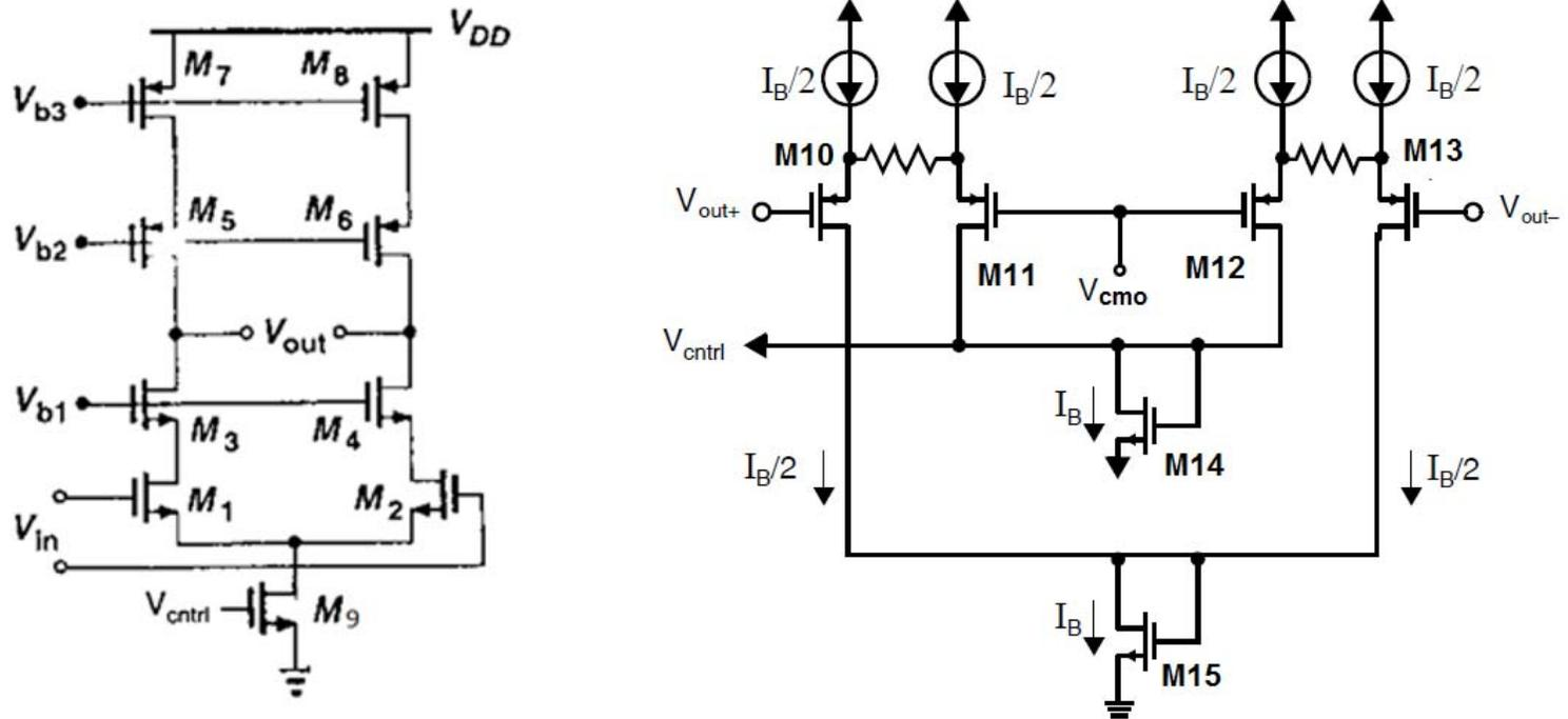
A continuous-time CMFB circuit that can accommodate increased output swing.
