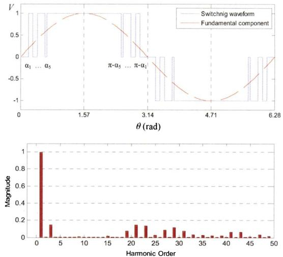
Figure 2: A typical selective harmonic elimination ( $5^{\text{th}}$ ,  $7^{\text{th}}$ ,  $11^{\text{th}}$ , and  $13^{\text{th}}$ ) based on quarter-cycle symmetry: the waveform and its harmonic spectra.
