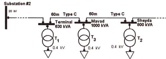
Figure 7: Single-line diagram of the distribution network under study.
