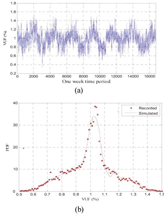
Figure 11: (a) The VUF% variation over the one week period at the low-voltage side of T3 obtained using the proposed simulation method, and (b) comparing the PDFs of VUF% obtained from field measurements (dotted line) and the proposed algorithm (solid line).
