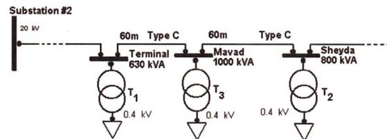
Figure 7: Single-line diagram of the distribution network under study.
