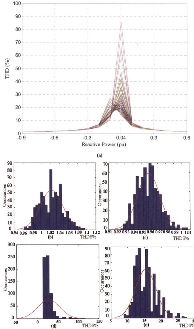
Figure 12: (a) Penetrated THDS due to the 5<sup>th</sup>, 7<sup>th</sup>, 11<sup>th</sup>, 13<sup>th</sup>, 17<sup>th</sup> and 19<sup>th</sup> harmonics under various VUF% and reactive power obtained from Monte Carlo Simulation. (b)-(e) distributions of the THDS corresponding to the reactive power loadings of -0.8 P.U., -0.9 P.U., 0.04 P.U. and -0.1 P.U., respectively.
