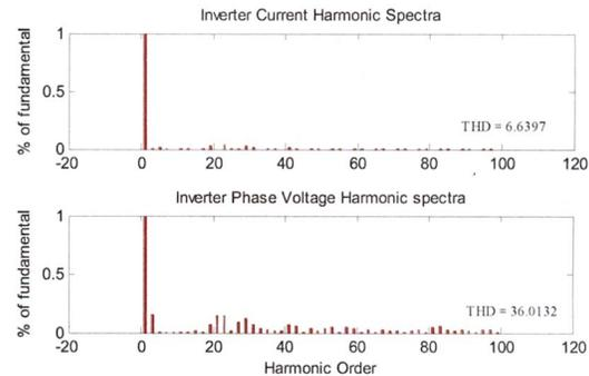
Figure 6: Harmonic spectra of  $V_{th}$  and  $I_{inv}$ .
