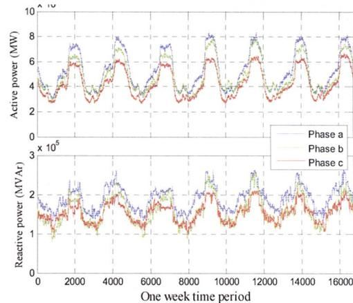
Figure 8: Recorded three-phase active and reactive powers by data logger that is installed at 400 V substation of Mavad.
