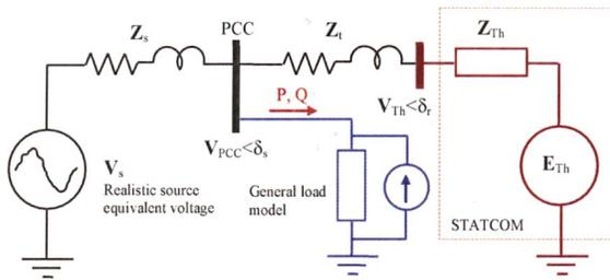
Figure 3: Suggested three-phase modeling for a STATCOM in the harmonic-domain that is connected to a distribution substation.
