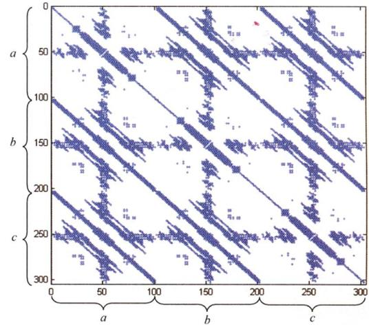
Figure 4: STATCOM equivalent impedance matrix structure implying the phases  $a$ ,  $b$  and  $c$  components cross coupling for harmonics bigger than 0.02 P.U. up to 50<sup>th</sup>.
