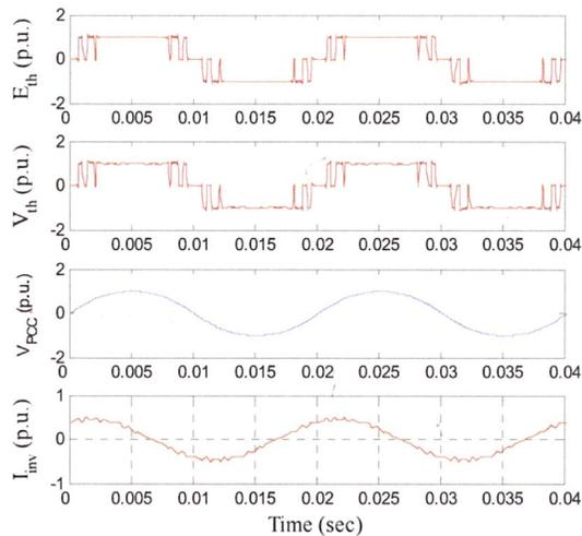
Figure 5: Simulations of the model (6) under balanced condition when STATCOM supplies 1 P.U. reactive power to the PCC; pictures from the top one are the Thevenin voltages ( $E_{th}$  and  $V_{th}$ ), the PCC voltage at phase  $a$  ( $V_{PCC}$ ), and the converter current at phase  $a$  ( $I_{inv}$ ) all in P.U.
