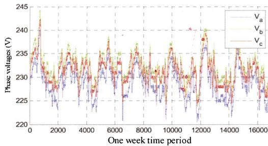
Figure 9: Measured phase voltages of the transformer T3 (Mavad) during a week.
