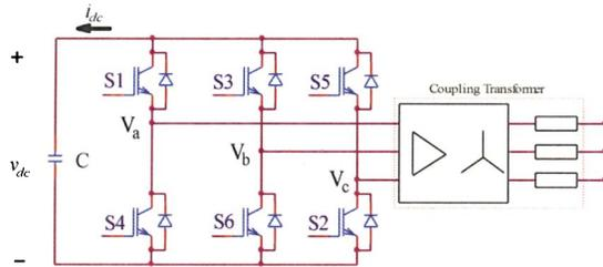
Figure 1: Three-phase voltage source converter connected to the power system through a transformer.
