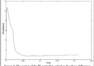
Figure 4: The output of the PI controller, which is the phase difference between the PCC voltage and the converter output voltage.
