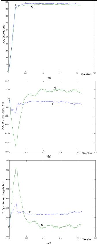
Figure 7: Active and reactive power of (a) the load, (b) the compensator (STATCOM), and (c) the source after compensation.
