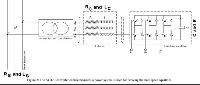
$\mathbf{u}(t)$  is the three-phase applied voltages [4], [8]. State-space model (1) is described with block 1 in Fig. 1 in which inputs include duty ratios as well as the applied three-phase voltages. Also, the output shows three-phase converter AC voltages. Duty ratios depend on the phase difference between the converter AC voltages and the applied voltages.
