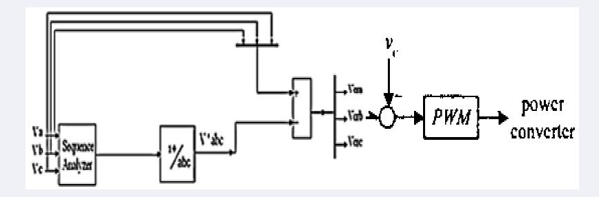
This controlled voltage source injects the compensation voltage needed to mitigate voltage sags and total harmonic distortion into the utility. Now the control algorithm based on the generalized theory of instantaneous power definitions generates satisfactory reference signals for the SAPF in the presence of a balanced linear load; therefore, the injecting current of the SAPF would be led to a sinusoidal wind turbine-end currents.
