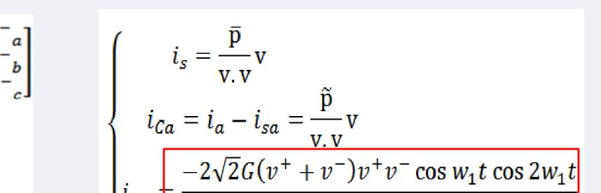
The control algorithm based on the generalized theory of instantaneous power definition not only generates wrong references for the SAPF (injecting a distorted current into the distribution system) but also causes the supply current distortion. So the situation could be much worse in the presence of wind turbine voltage asymmetry and harmonics.
