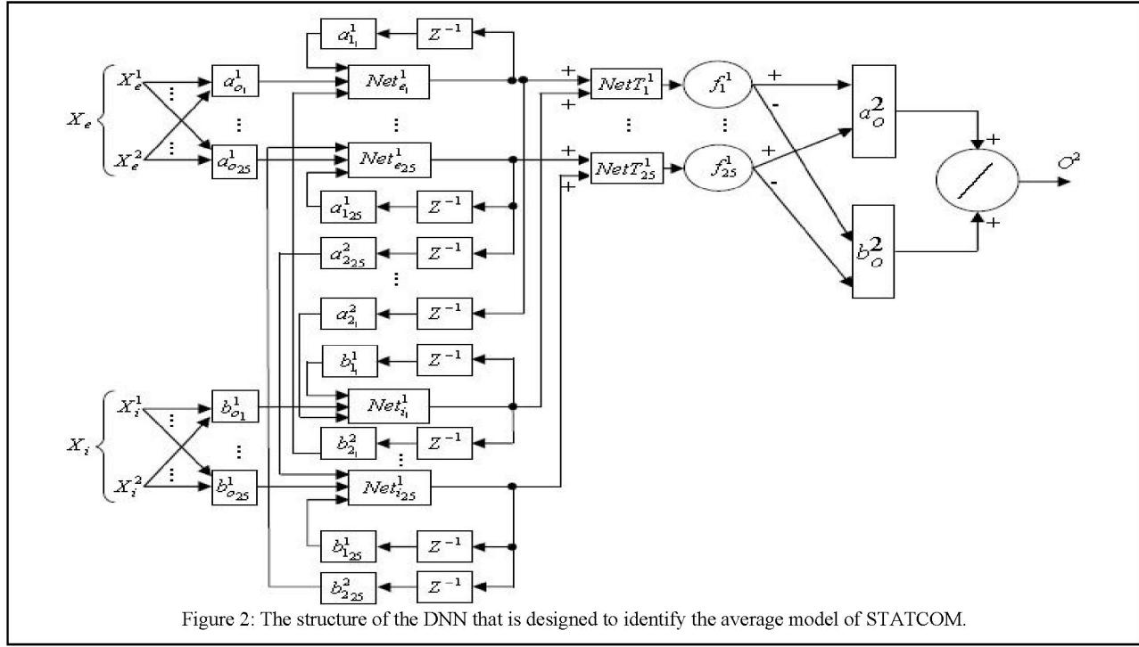
Figure 2: The structure of the DNN that is designed to identify the average model of STATCOM.
