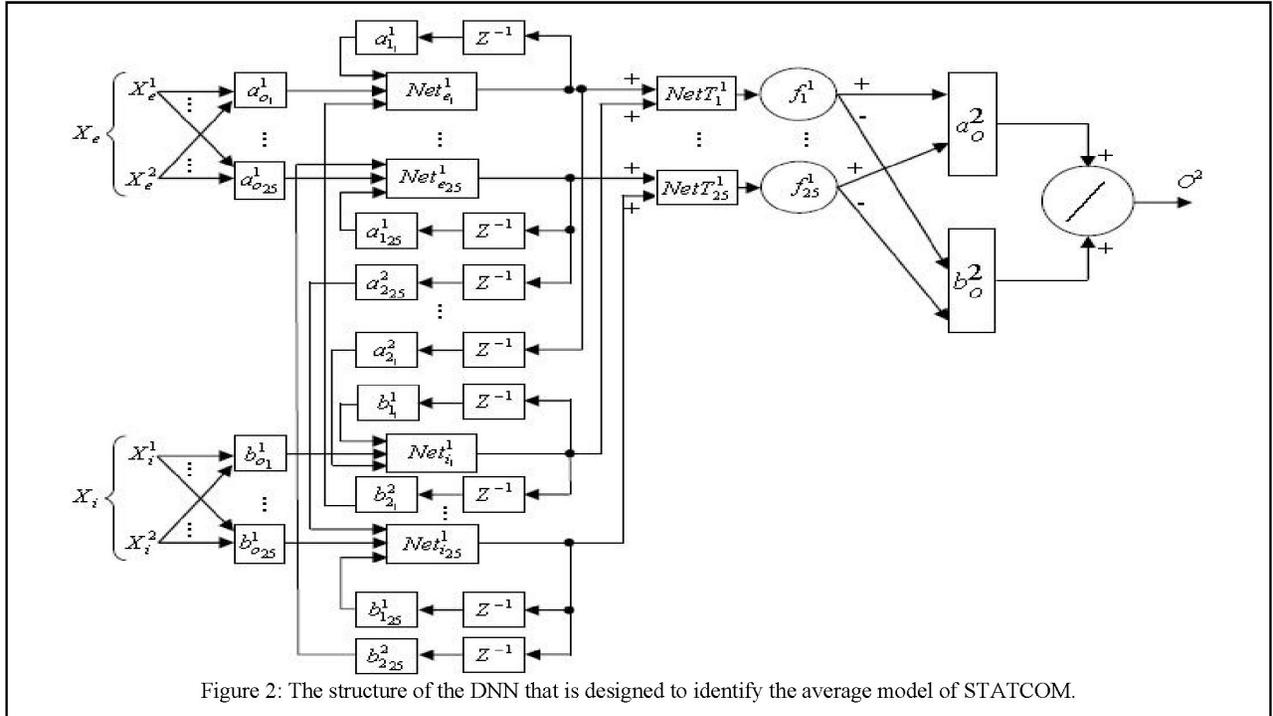
Figure 2: The structure of the DNN that is designed to identify the average model of STATCOM.
