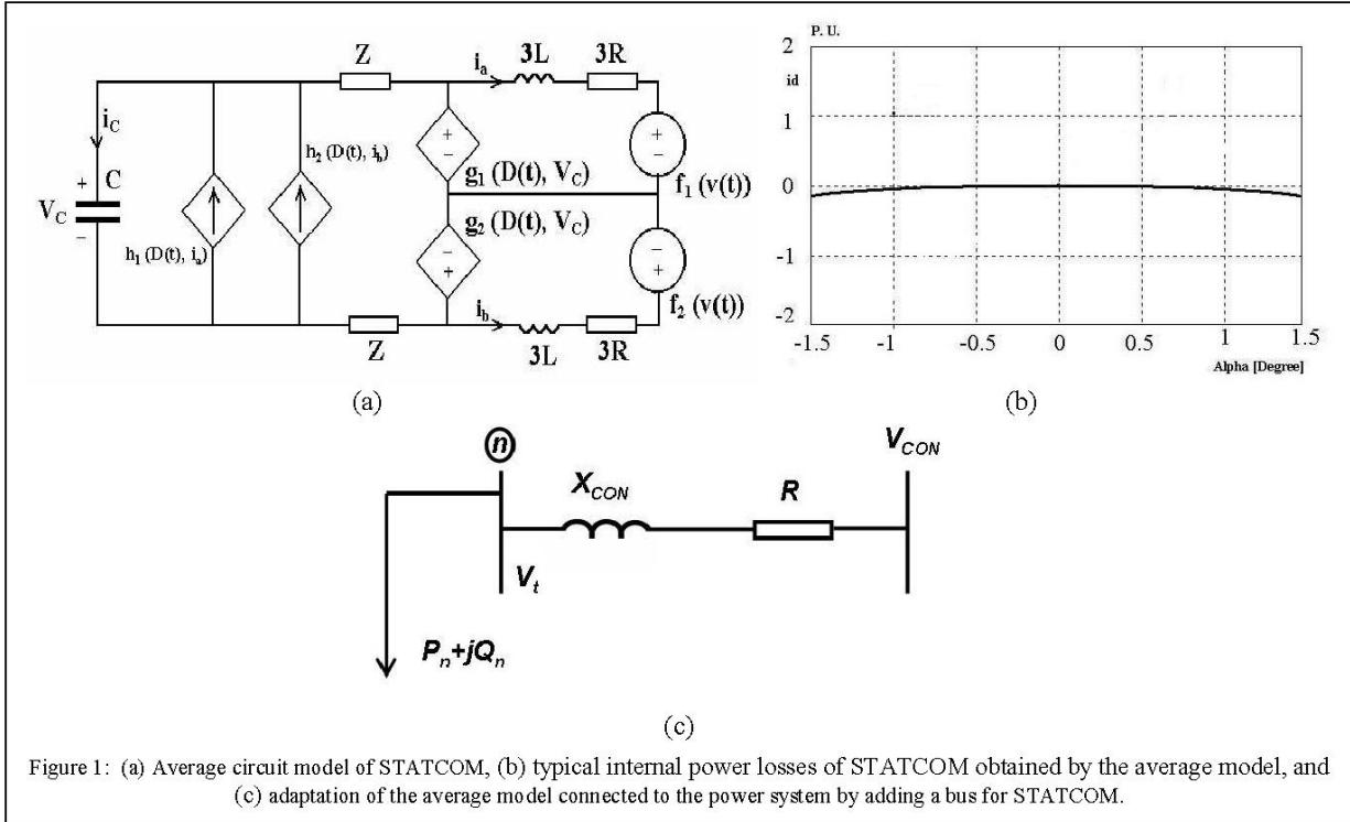
Figure 1: (a) Average circuit model of STATCOM, (b) typical internal power losses of STATCOM obtained by the average model, and (c) adaptation of the average model connected to the power system by adding a bus for STATCOM.
