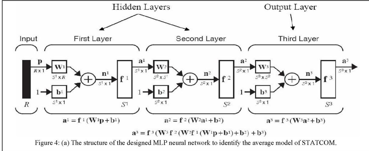
Figure 4: (a) The structure of the designed MLP neural network to identify the average model of STATCOM.
