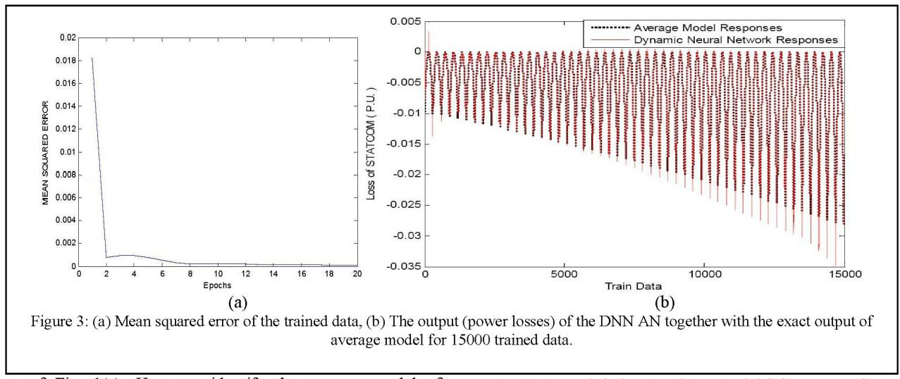
Figure 3: (a) Mean squared error of the trained data, (b) The output (power losses) of the DNN AN together with the exact output of average model for 15000 trained data.
