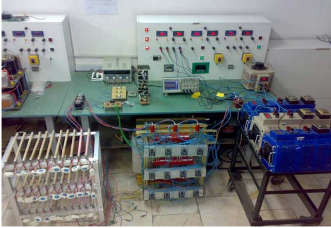
Fig. 11. Developed modular design of the LBT for practical examination of the four various cases.
