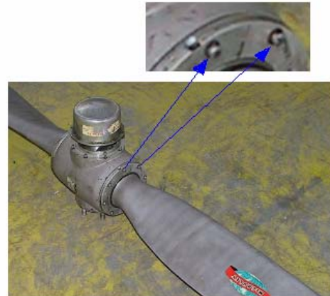
Figure 4. Sample control points used to register coordinate systems of measurements for both blades
