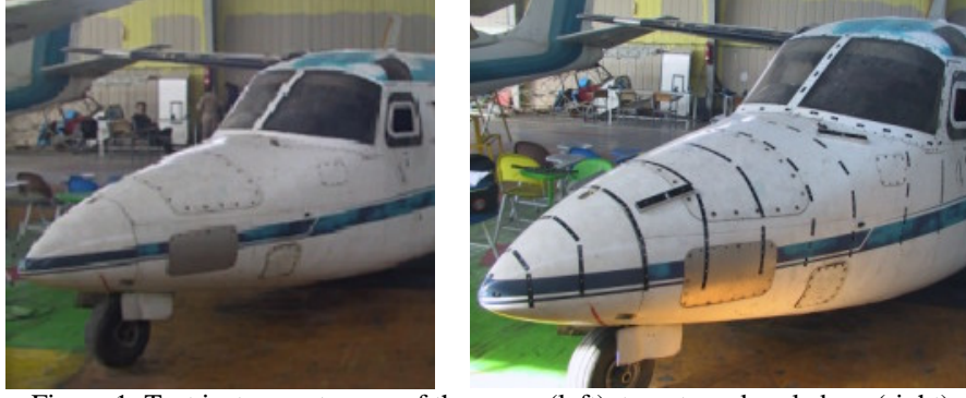
Figure 1: Test instruments: one of the noses (left), targets and scale bars (right)
