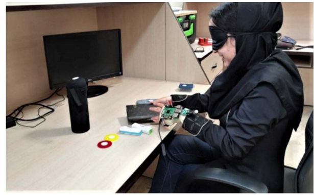
Fig. 7. Participants perform test 1 on eight different objects. The goal is to identify these objects, and in case of an unknown tag, they enter new voice recordings with the help of a supervisor.
