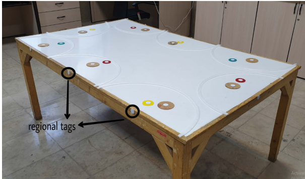
Fig. 6. Setup 4. A rectangular table was divided up into 8 sections, labeled with RFID tags by alphabet characters. There are two or three disks inside each region.
