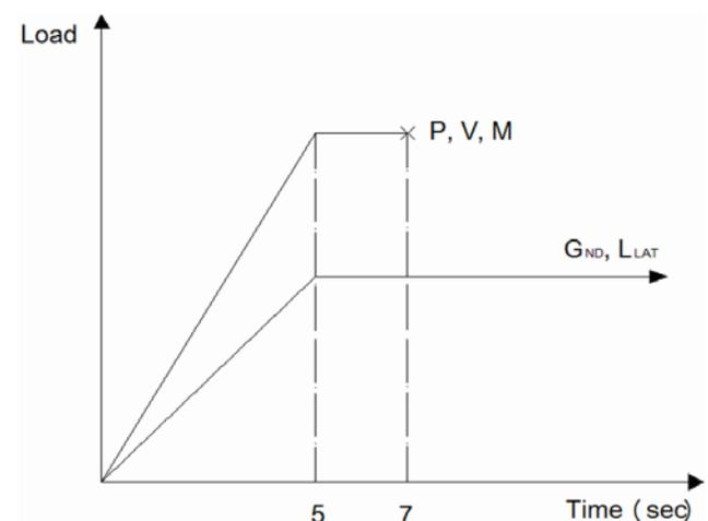
**Figure 2.** Applying dynamic loads for nonlinear dynamic procedure.
