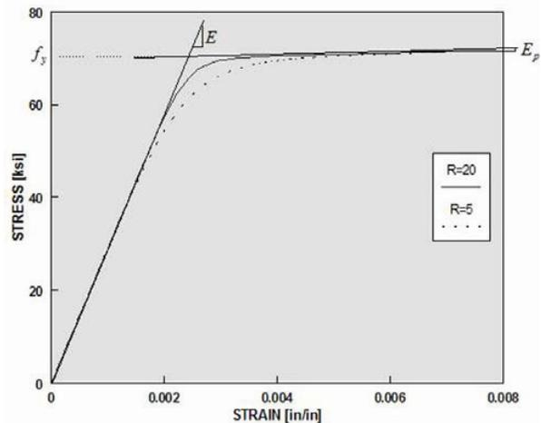
**c.** Material Parameters of Monotonic Envelope.
