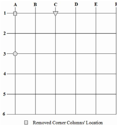
**Figure 3.** Notionally removed corner column for AP analysis.
