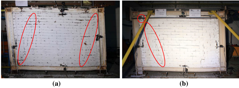
Fig. 7 Crack formation and failure modes at the end of the test a Specimen DL, b Specimen CL
