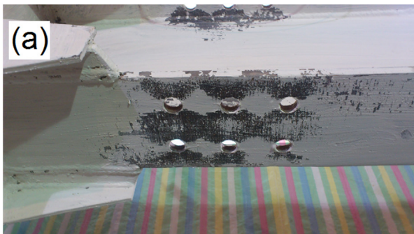
Fig. 26. Connection condition; a) at the interstory drift angle of 0.04 rad; b) at the interstory drift angle of 0.06 rad.
