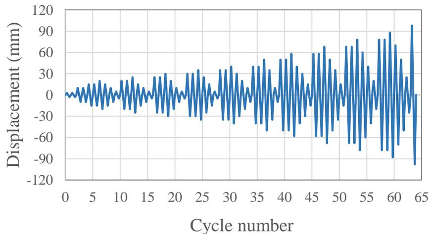
Figure 5. Cyclic displacement protocol.
