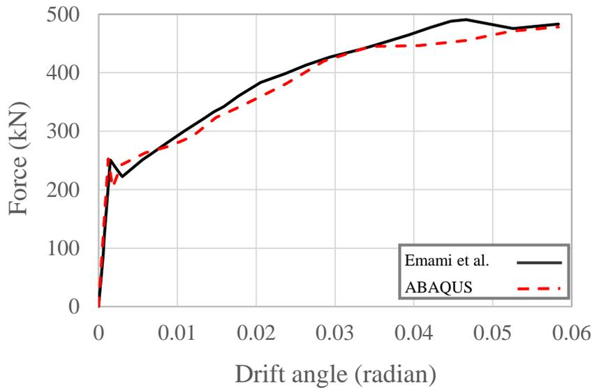
Figure 7. Backbone curve of the horizontally corrugated-web shear wall.
