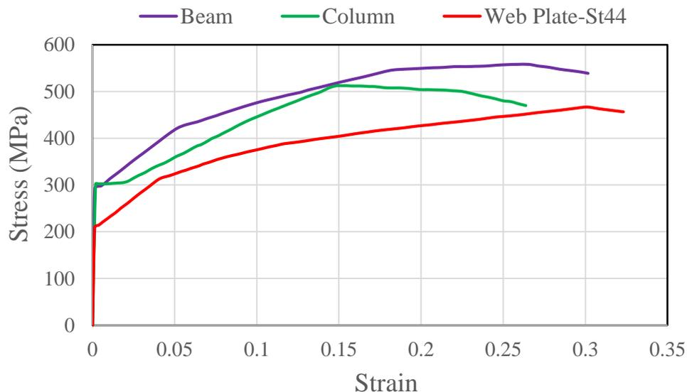
Figure 3. Uniaxial tensile behavior of used steels in members.
