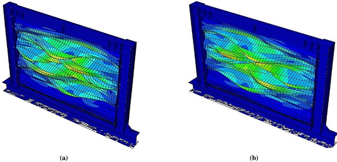
Figure 4. Eigen buckling analyses results of the H-CSPSW: a) First buckling mode shape; b) Second buckling mode shape.
