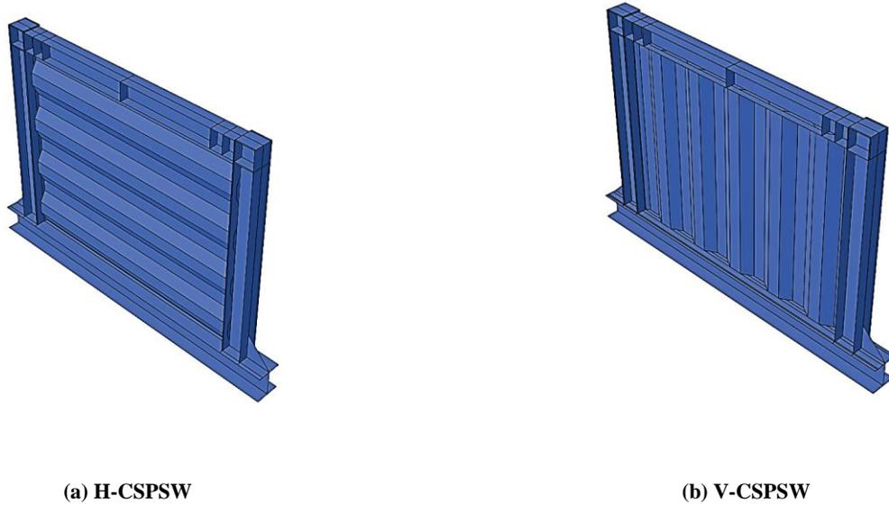
Figure 2. Finite element models of the corrugated steel plate shear walls.
