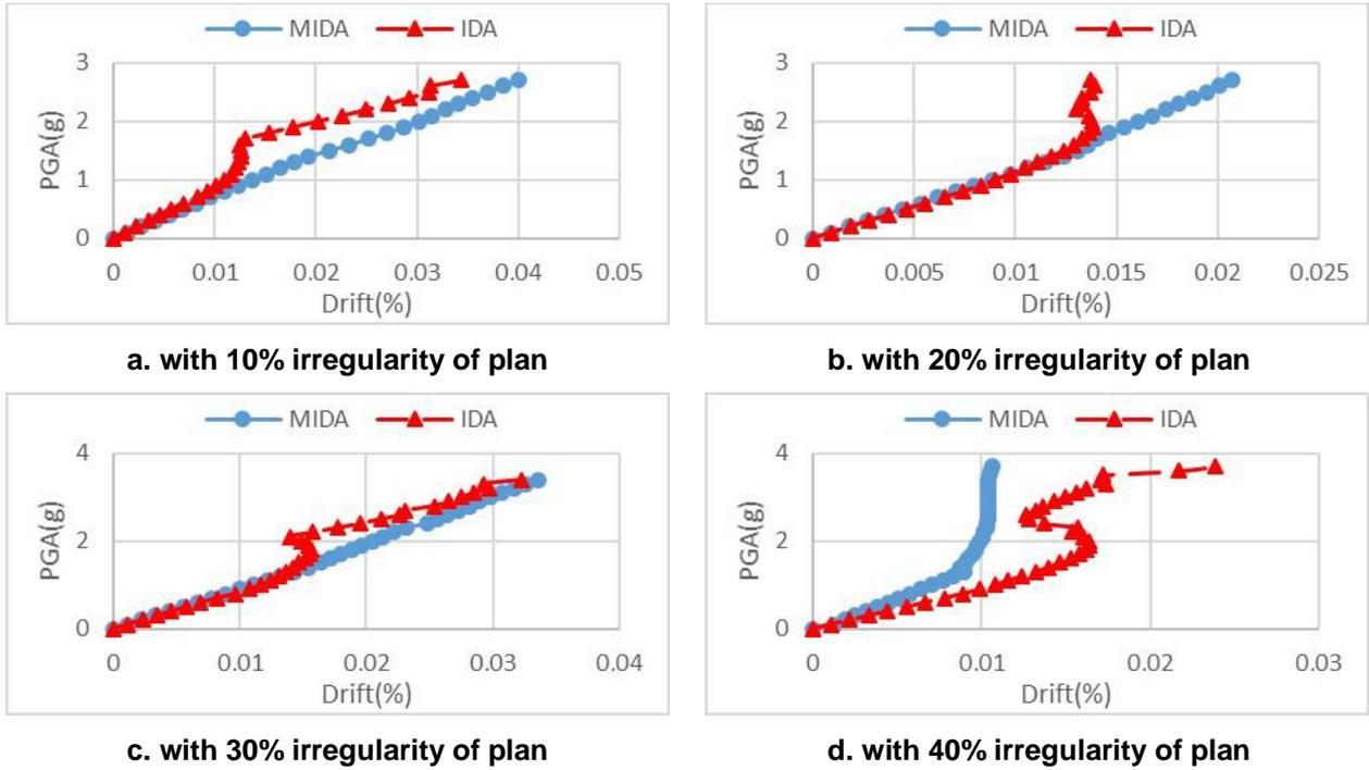
**Figure 7. Comparison of roof drift from IDA and MIDA methods in 12-storey structures for record No.1 in near field records.**
