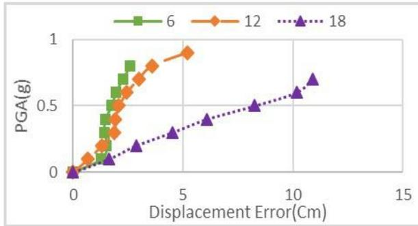
c. In structures with 20% irregularity on Y-Direction
