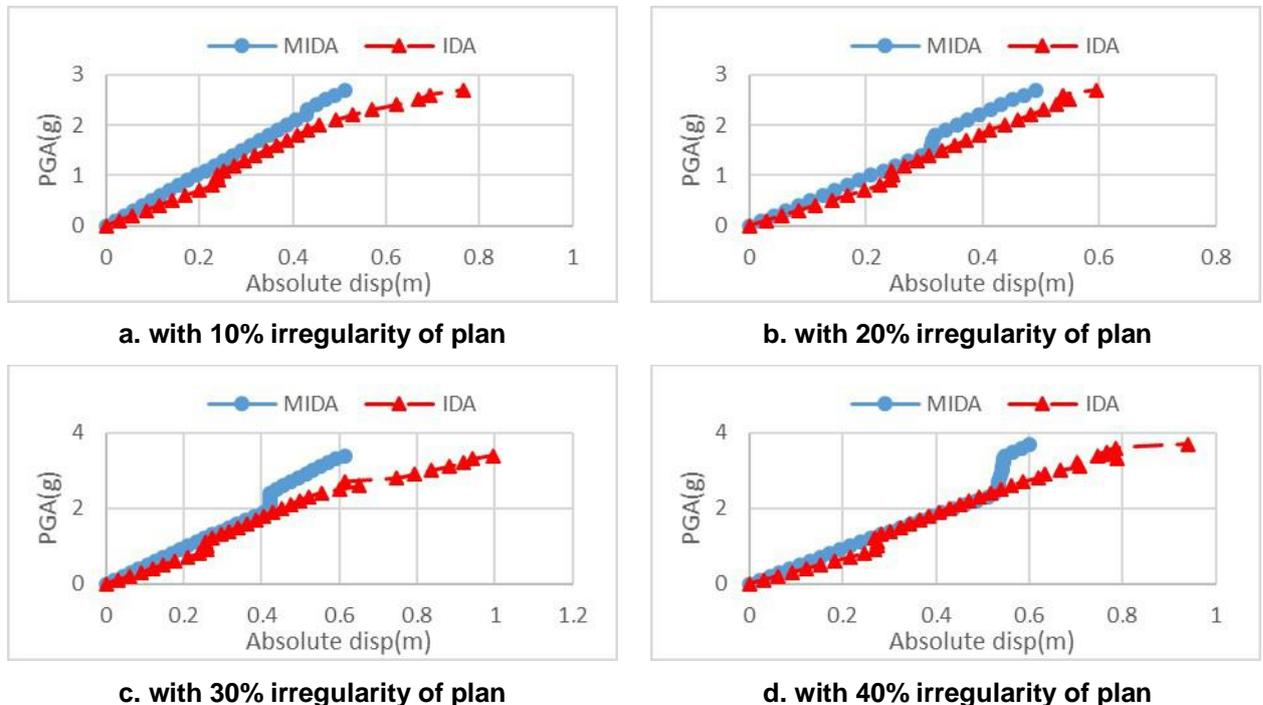
**Figure 6. Comparison of roof displacement from IDA and MIDA methods in 12-storey structures for record No.1 in near field records.**
