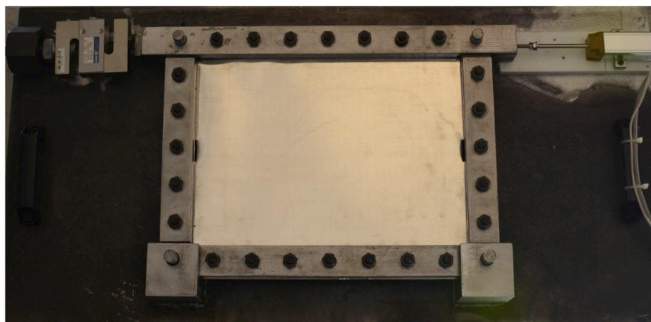
Fig. 7. Small-scale specimen test setup (NCR = 10%).
