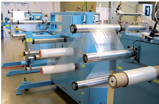
Fig 23. Membrane production for PEM fuel cell
