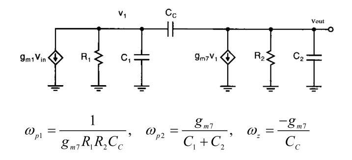
•As  $g_{m7}$  increases, the separation between the first and second poles increase. •Increasing  $C_C$  moves the dominant pole to a lower frequency without affecting the second pole.
