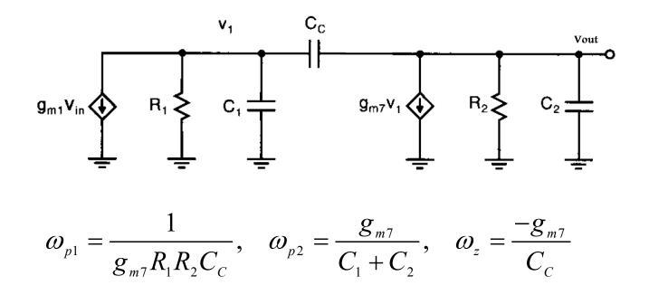
•A problem arises due to the right-half-plane zero,  $\omega_z$ . It introduces negative phase shift (phase lag).
