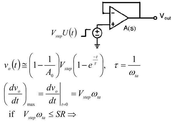
The circuit has only the linear settling - time.
