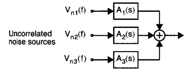
$$V_{no}^{2}(f) = \sum_{i=1, 2, 3} |A_{i}(j2\pi f)|^{2} V_{ni}^{2}(f)$$
