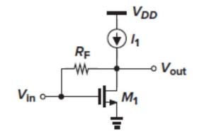
$$\overline{V_{n,in}^2} = \frac{\frac{4kT}{R_F} + 4kT\gamma g_m}{(g_m - \frac{1}{R_F})^2}$$
