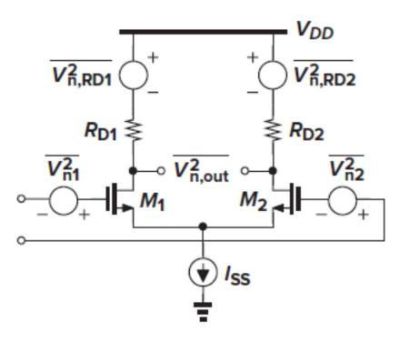
$$\overline{V_{n,in,tot}^2} = 8kT\left(\frac{\gamma}{g_m} + \frac{1}{g_m^2 R_D}\right)$$
