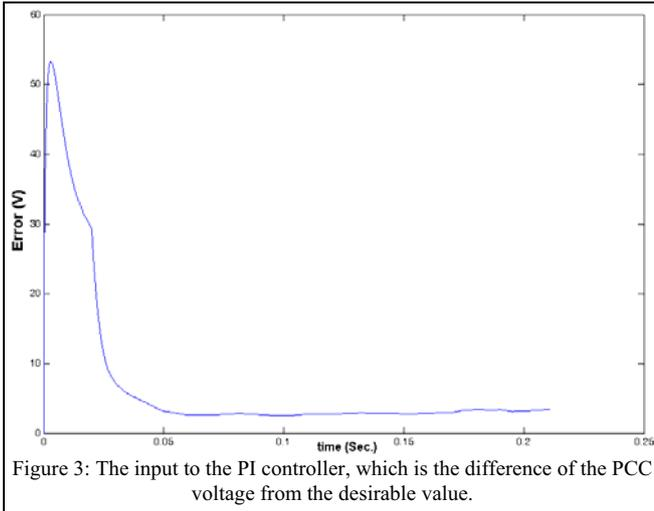
Figure 3: The input to the PI controller, which is the difference of the PCC voltage from the desirable value.
