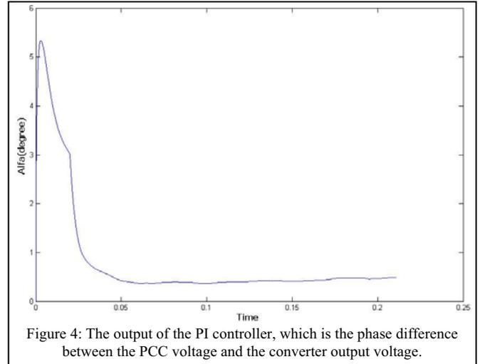
Figure 4: The output of the PI controller, which is the phase difference between the PCC voltage and the converter output voltage.
