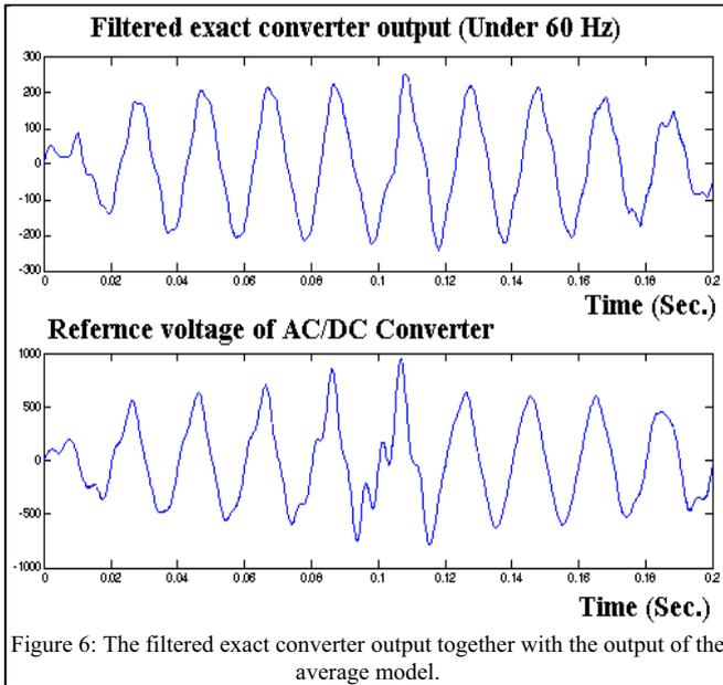
Figure 6: The filtered exact converter output together with the output of the average model.
