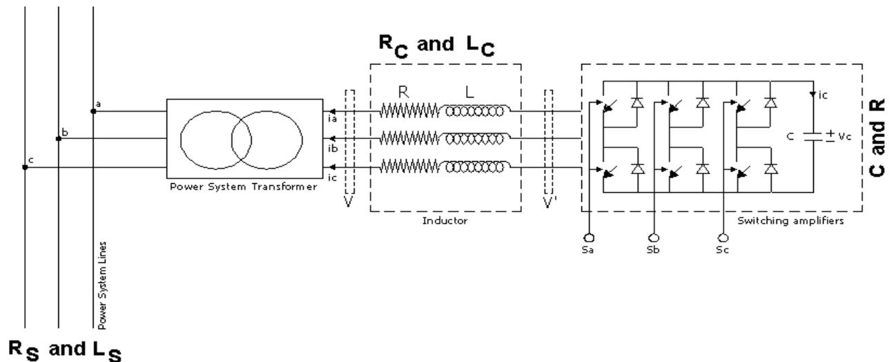
Figure 2: The AC/DC converter connected across a power system is used for deriving the state space equations.
