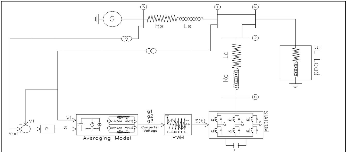
Figure 1: The proposed closed-loop control of STATCOM that contains three main blocks; average model, controller and modulator.
