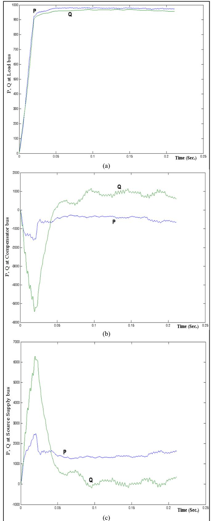
Figure 7: Active and reactive power of (a) the load, (b) the compensator (STATCOM), and (c) the source after compensation.
